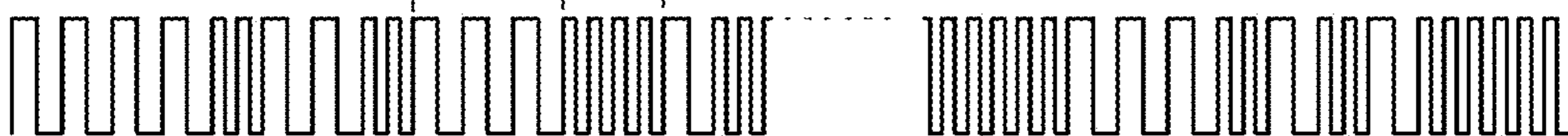
FIG. 24B AFTER FSK MODULATION
