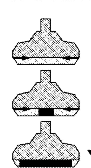
WHEN WIRE DIAMETER IS LARGER, GENERATION OF VOIDS DOES NOT PROMPTLY CAUSE FAILURE.
