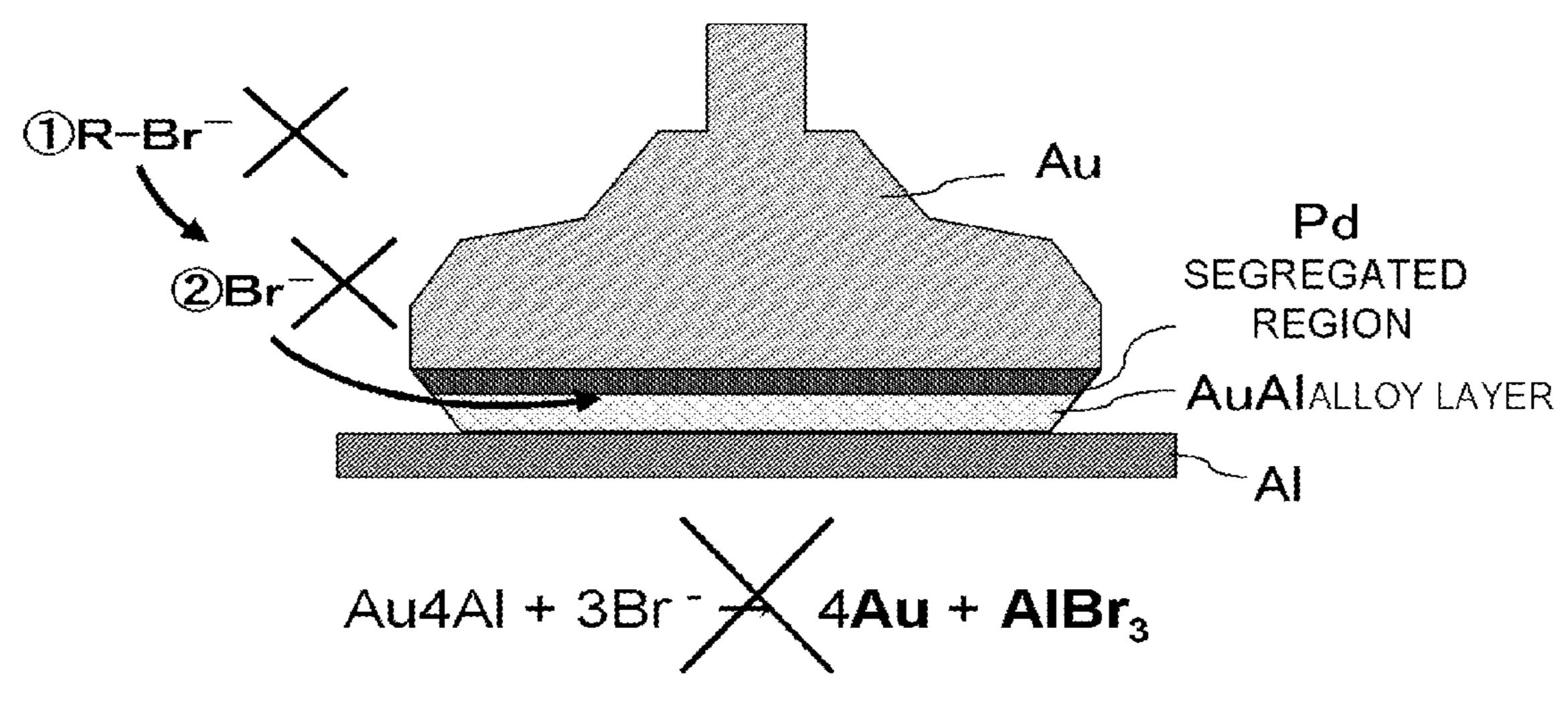
SINCE NO Br IS GENERATED, NO CORROSION BY ABOVE-DESCRIBED REACTION IS CAUSED. Nov. 19, 2013
