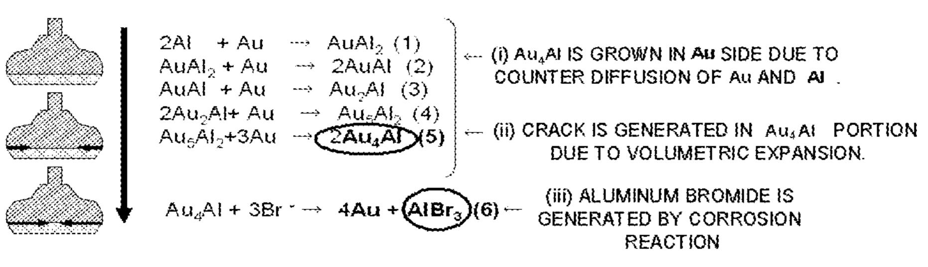
IT IS CONSIDERED THAT, SINCE AIBr. HAS LOWER MELTING POINT (97 DEGREE C), VOLUME THEREOF IS REDUCED IN AMBIENT TEMPERATURE. AND THUS VOIDS ARE GENERATED THEREIN.
