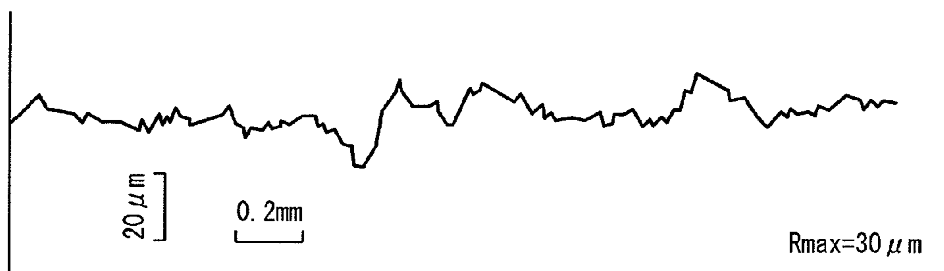
SURFACE ROUGHNESS AFTER REMOVAL OF AFFECTED LAYER (HYDROCHLORIC ACID 27~30°C)
