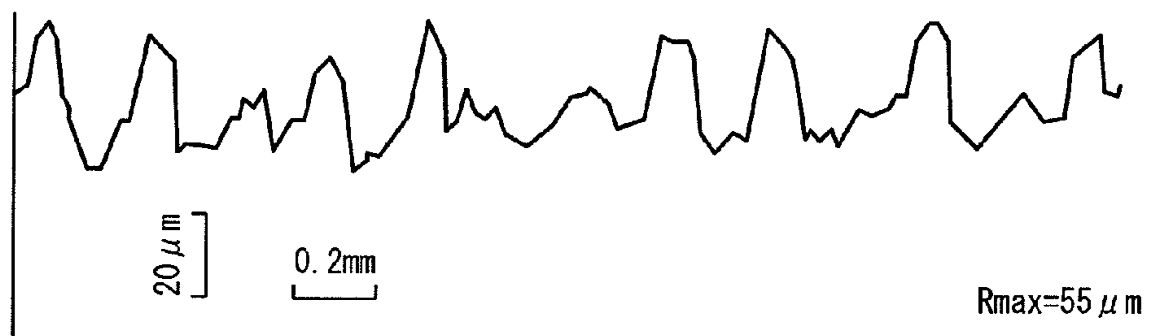
SURFACE ROUGHNESS AFTER REMOVAL OF AFFECTED LAYER (HYDROCHLORIC ACID 50°C)
