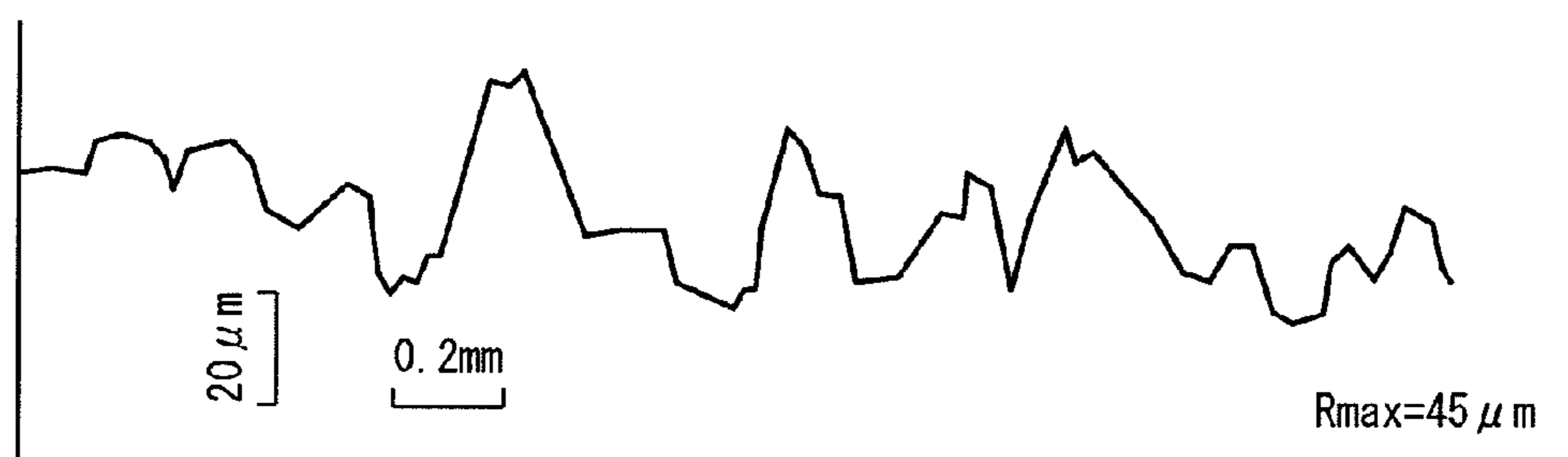
SURFACE ROUGHNESS PRIOR TO REMOVAL OF AFFECTED LAYER
