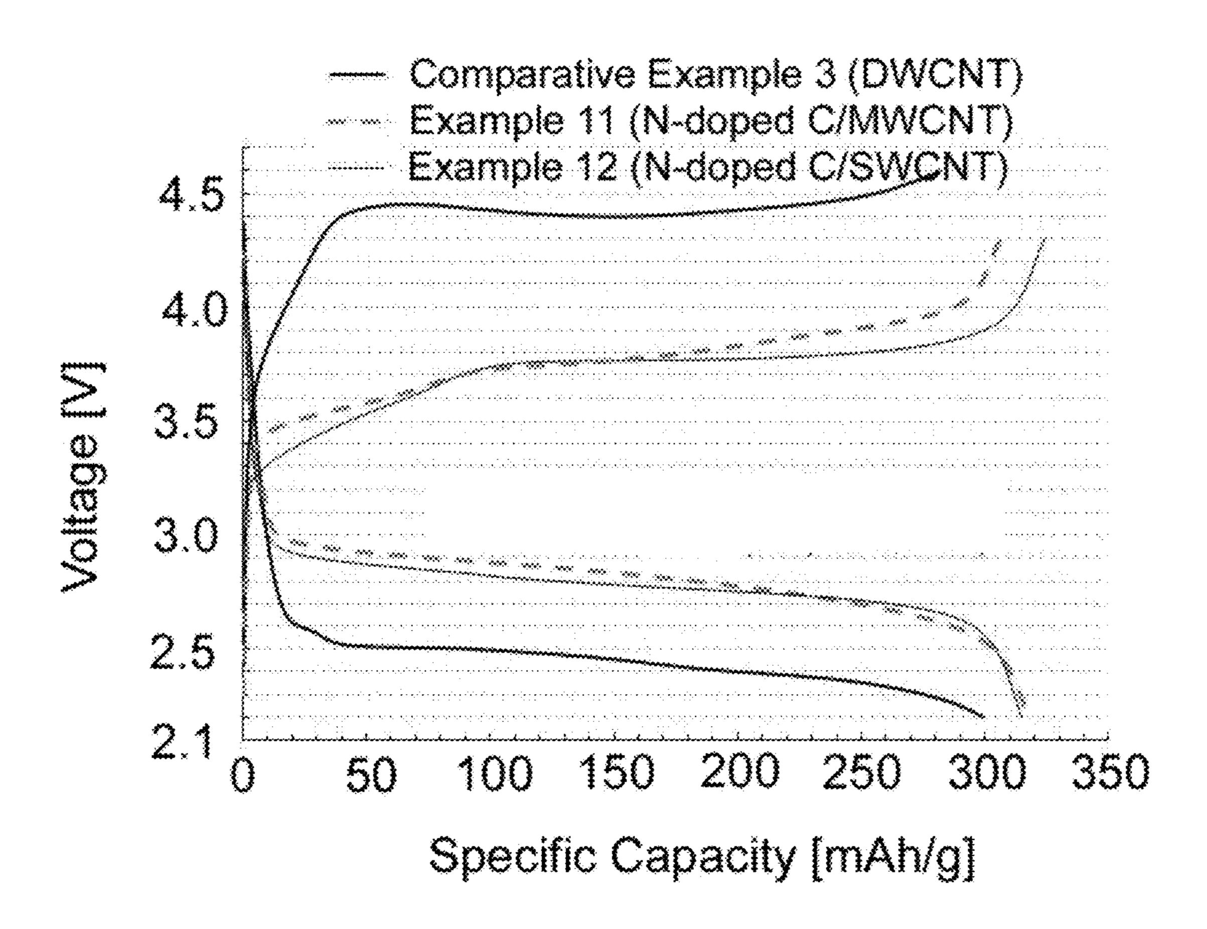
POROUS CARBONACEOUS COMPOSITE MATERIAL, POSITIVE ELECTRODE AND LITHIUM AIR BATTERY INCLUDING POROUS CARBONACEOUS COMPOSITE MATERIAL, AND METHOD OF PREPARING THE SAME
