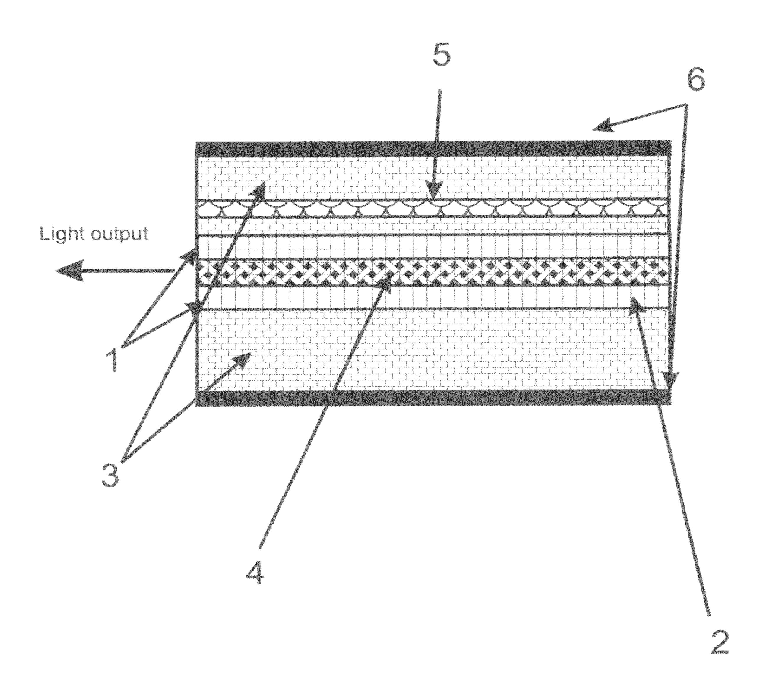
Fig. 1 Prior Art device: Distributed Feedback Laser
