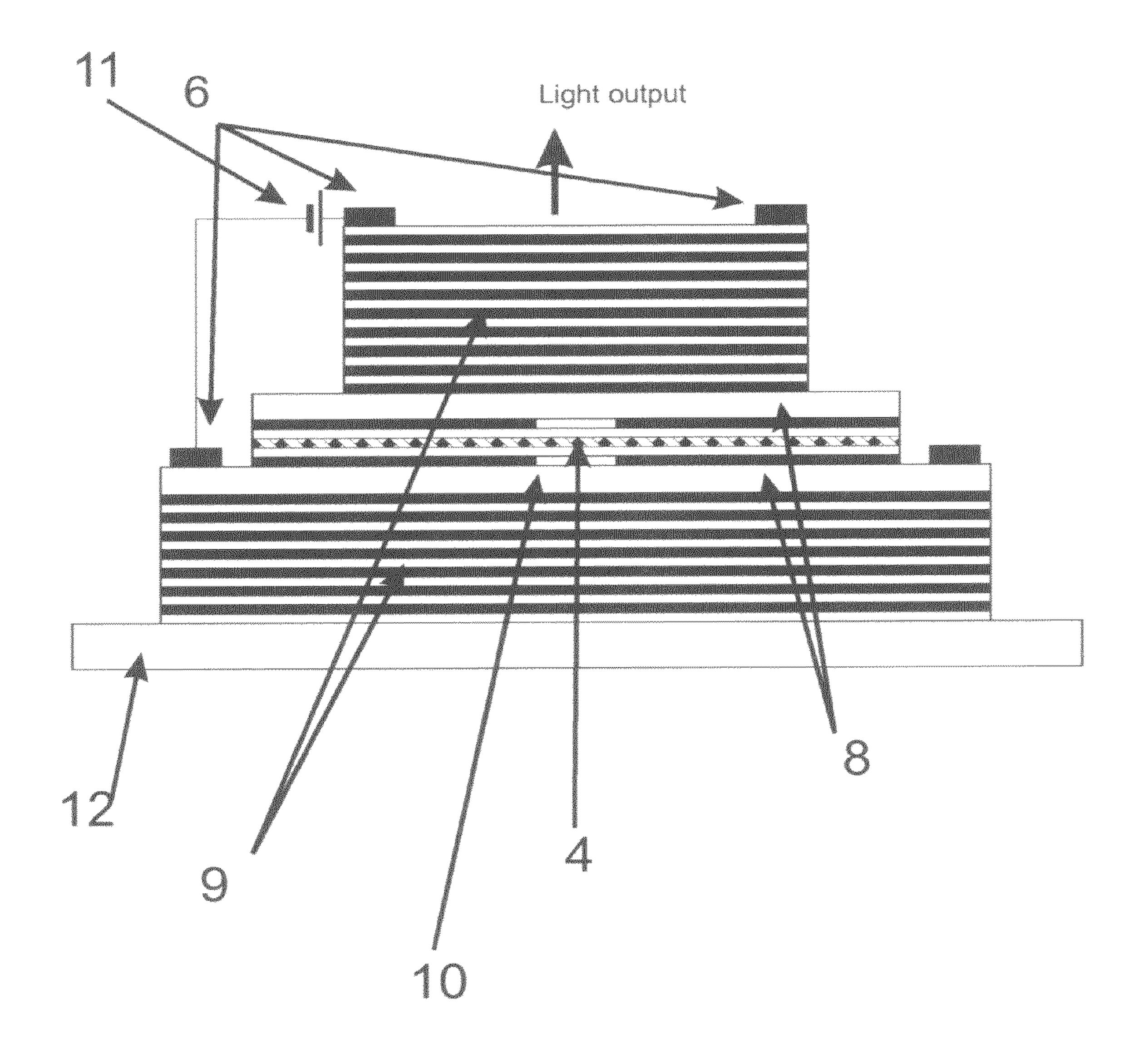
Fig. 2. Prior art device: vertical cavity surface-emitting laser
