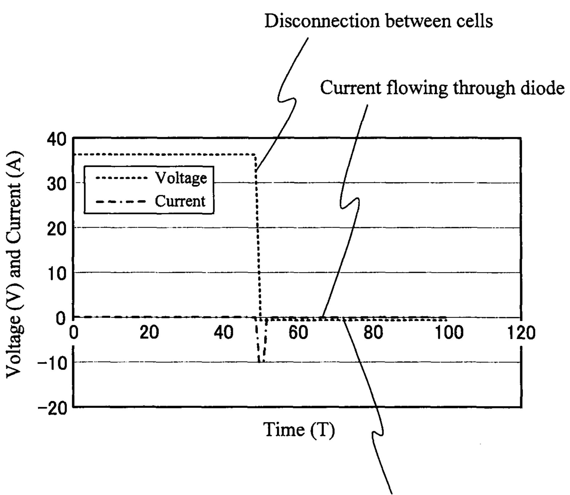
Voltage applied to battery voltage measurement circuit
