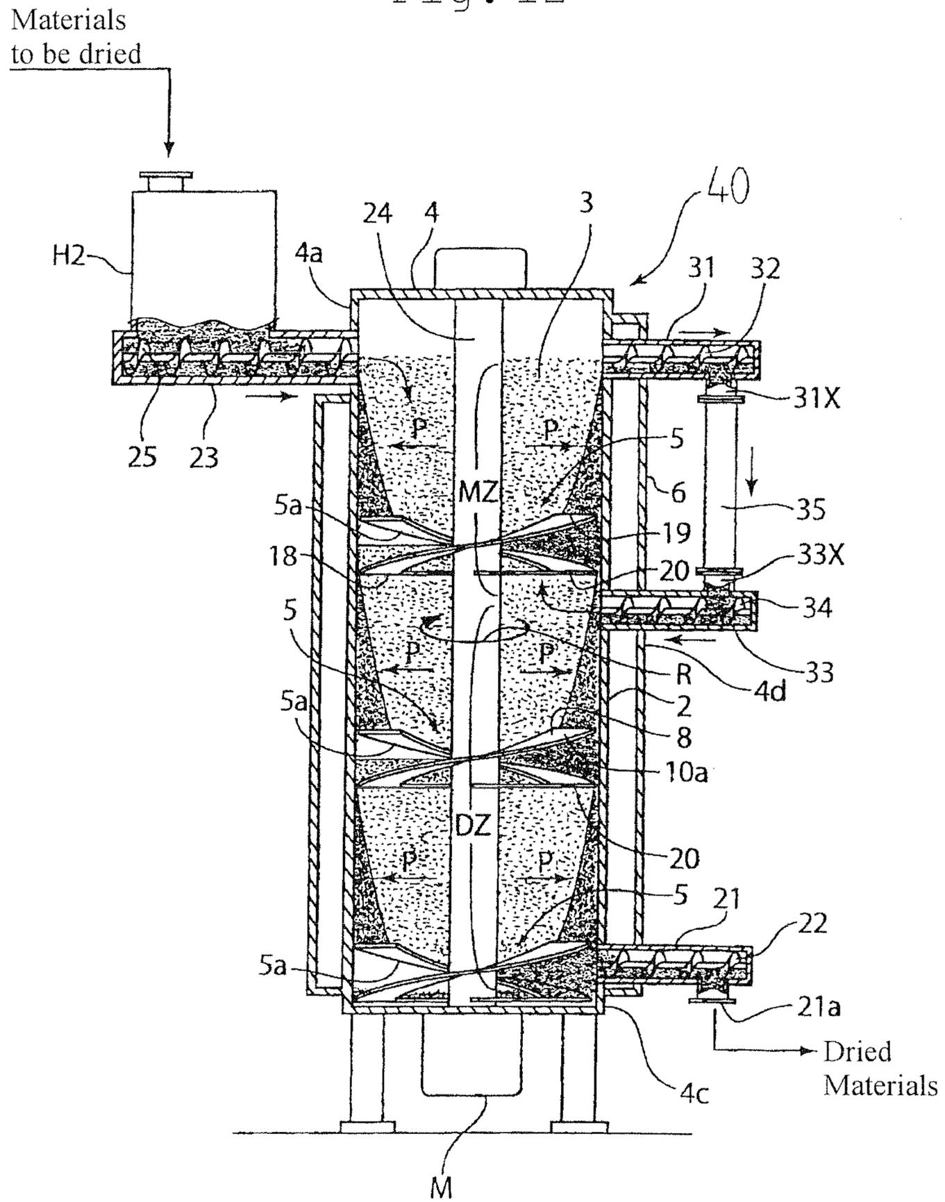
**CONTINUOUS DRYING APPARATUS**CROSS-REFERENCE TO RELATED
