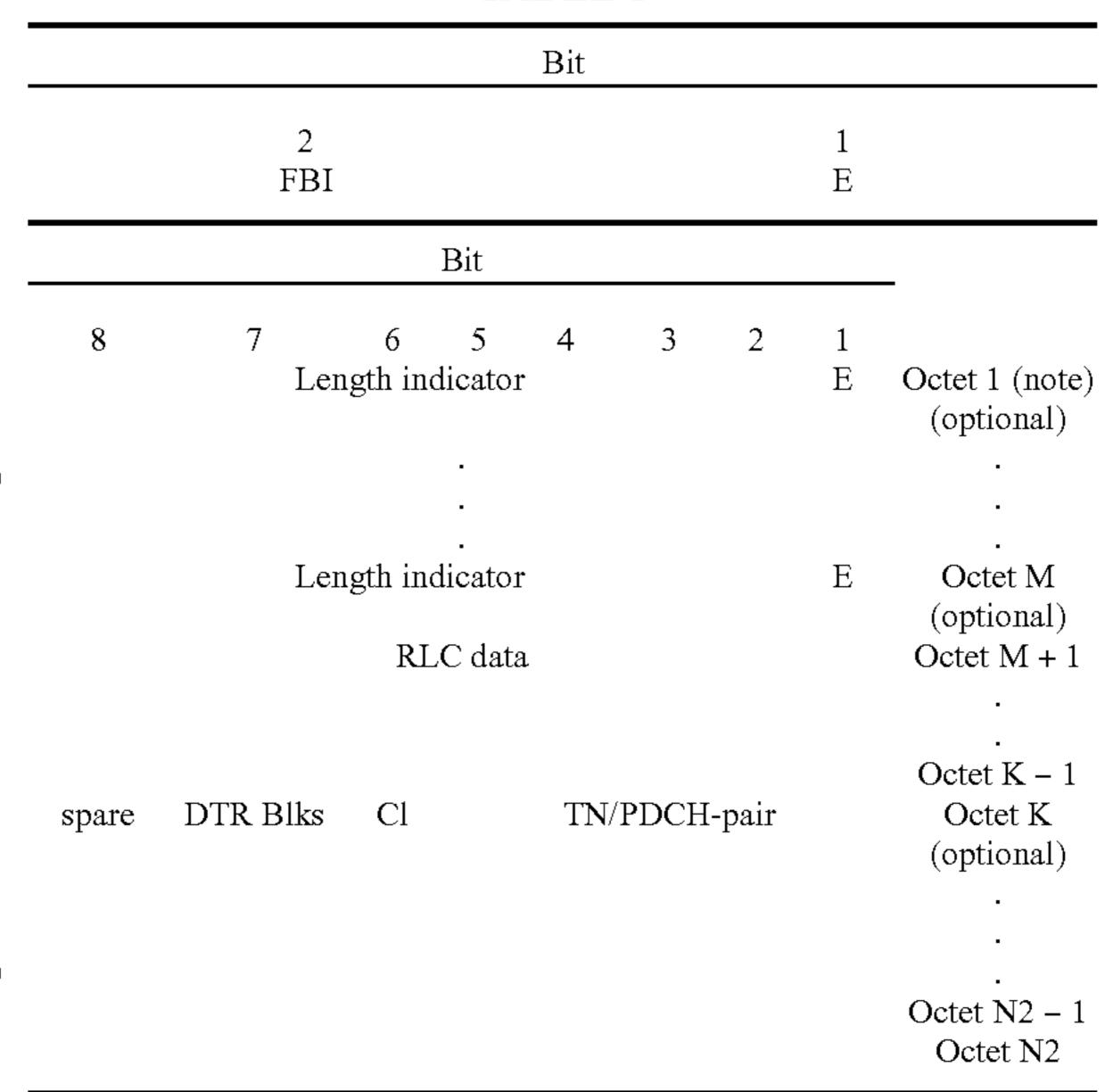
Referring to Table 1, the carrier ID (CI) field contains a identification of the carrier that may be encoded as DTR\_CI IE. The CI field can be used to indicate the carrier that the MS monitors when DTR is used. In that case, the timeslot or
