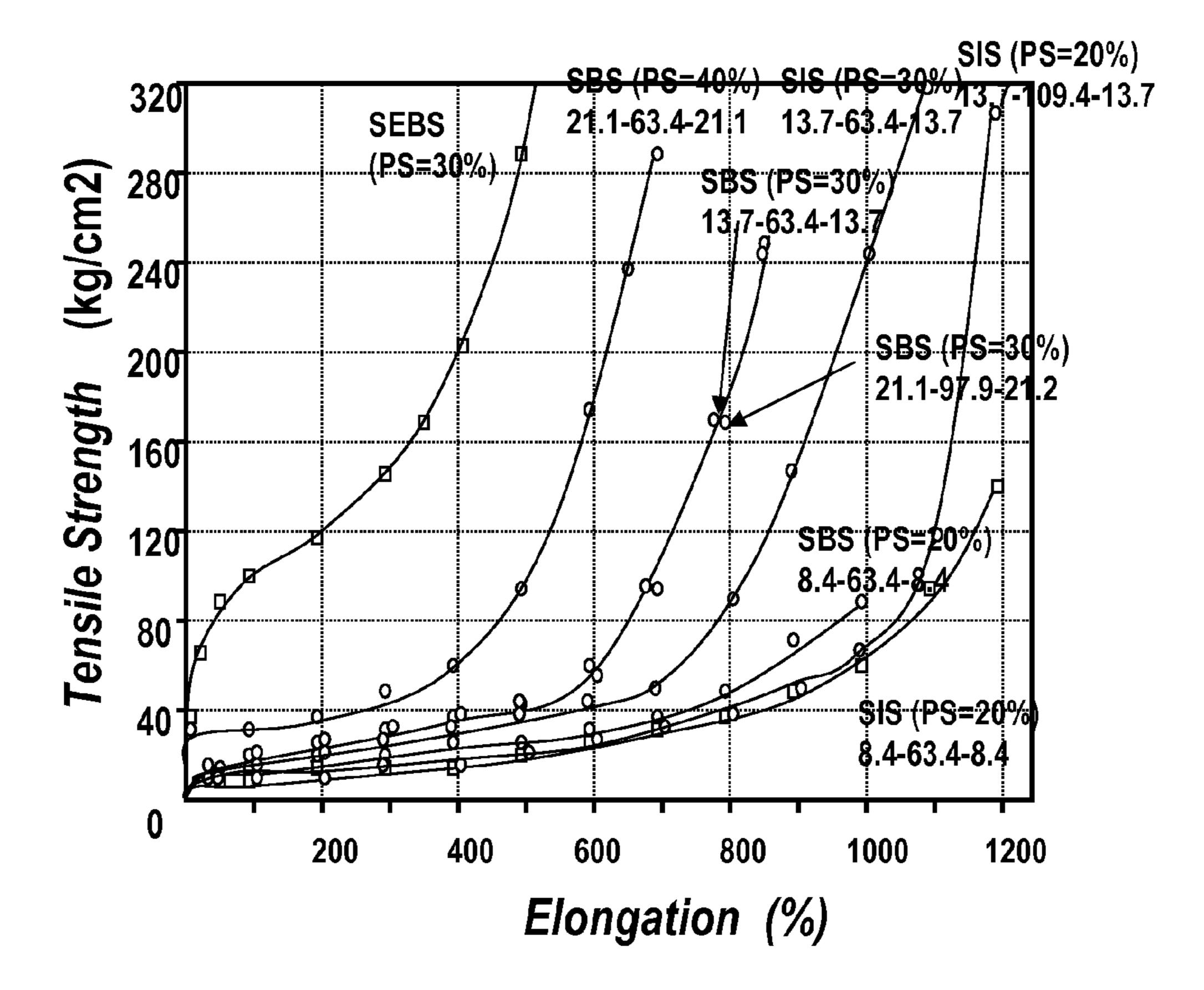
Tensile strength of SBS is greatly dependent on PS content.
