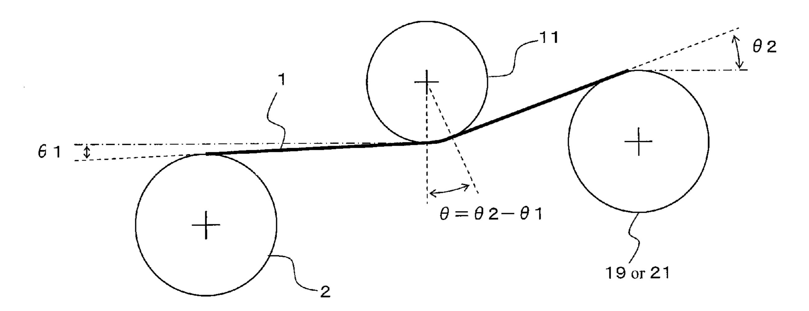
(b) In the case where a position of the upper surface of the guide roll 2 was higher than that of the lower surface of the coating rod 11
