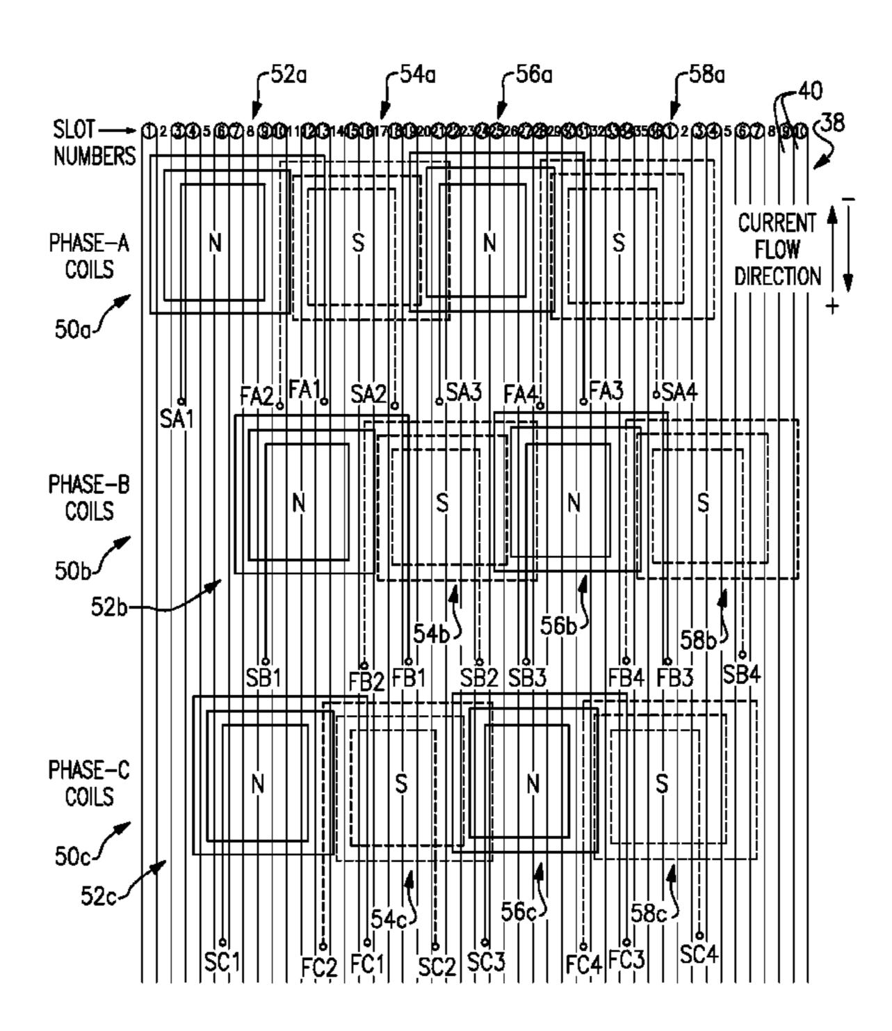
SC-DENOTES THE START OF THE COIL WIRE FC-DENOTES THE FINISH OF THE COIL WIRE N-DENOTES NORTH POLARITY S-DENOTES SOUTH POLARITY
