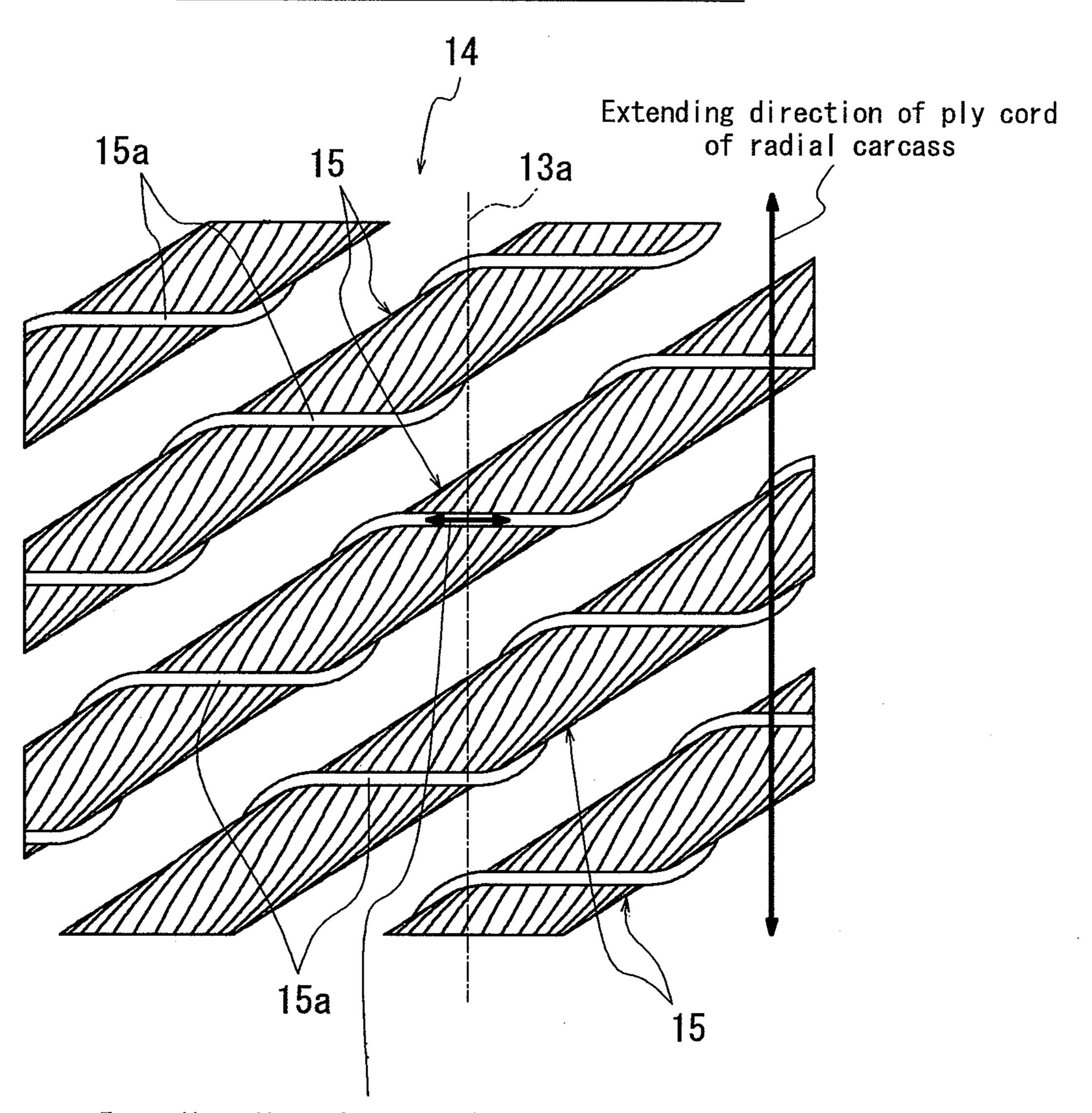
Extending direction of spiral filament 15a
