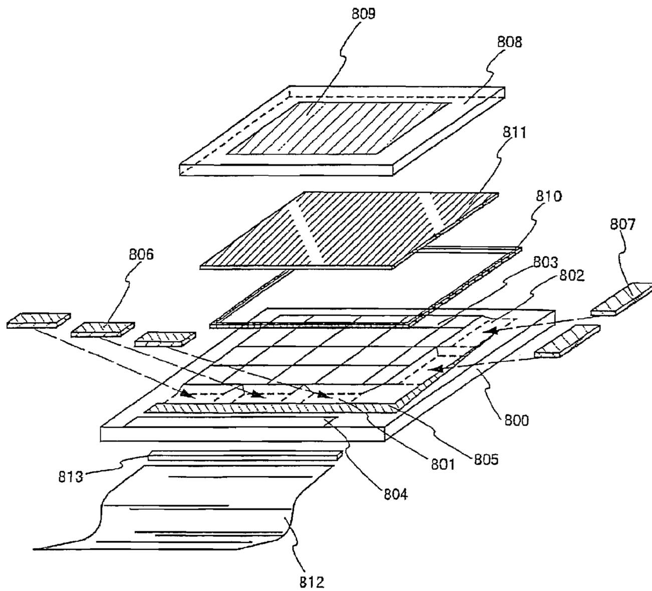
800: first substrate, 801: region for attaching IC chip (data line),
