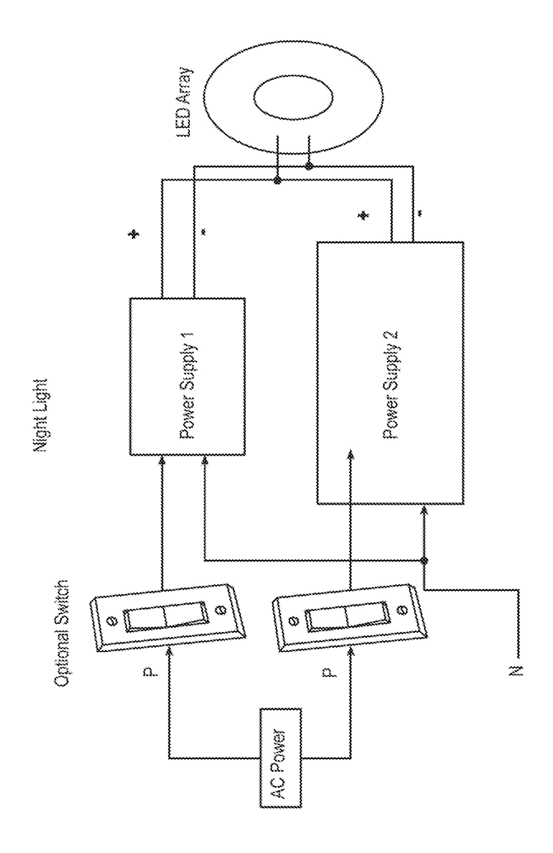
Driver #1 of lower current output will be driving the LED for night light mode, Driver #2 will drive the LED at full power mode.
