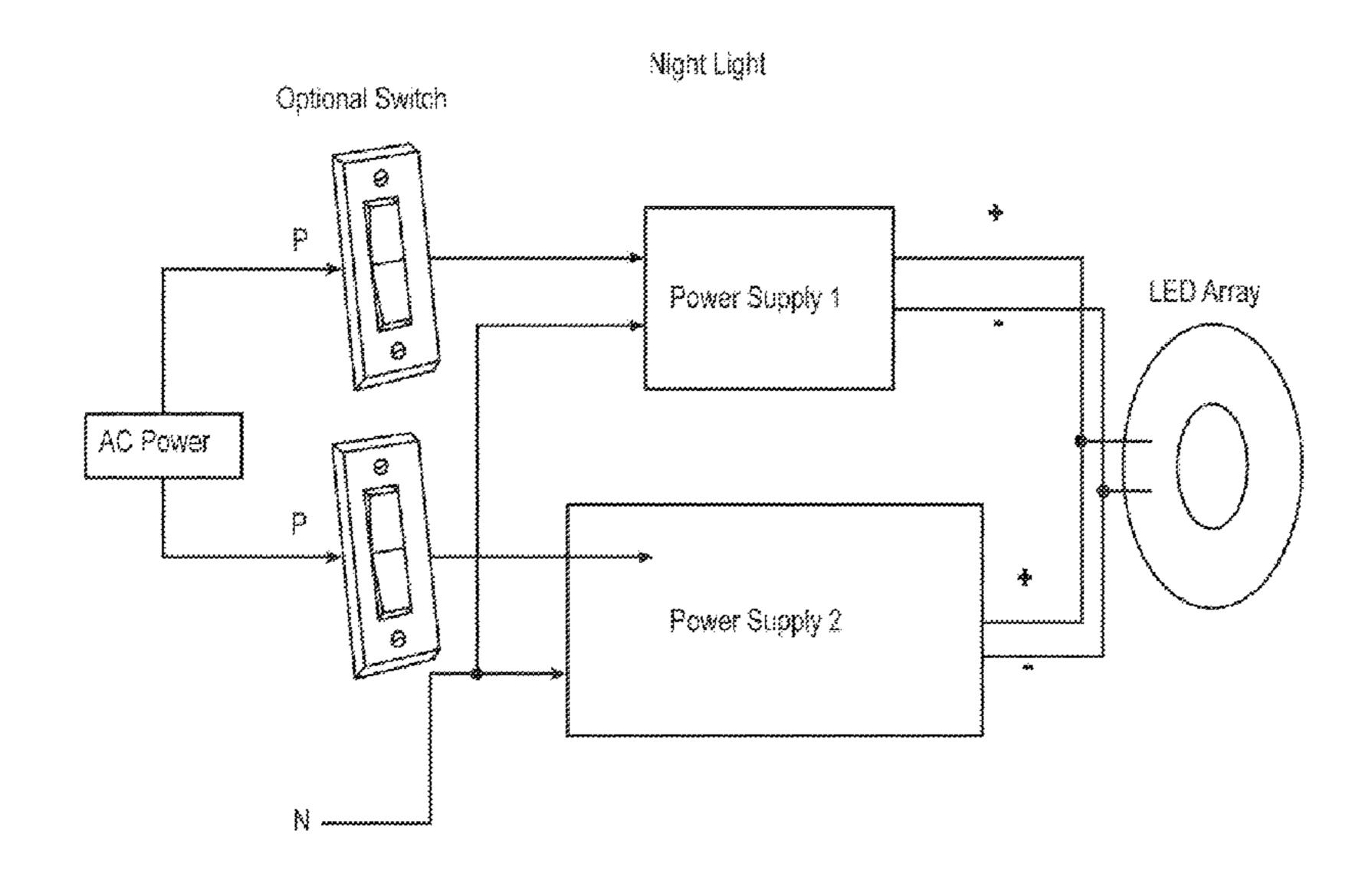
Oriver #1 of lower current output will be driving the LED for night light mode, Driver #2 will drive the LED at full power mode.
