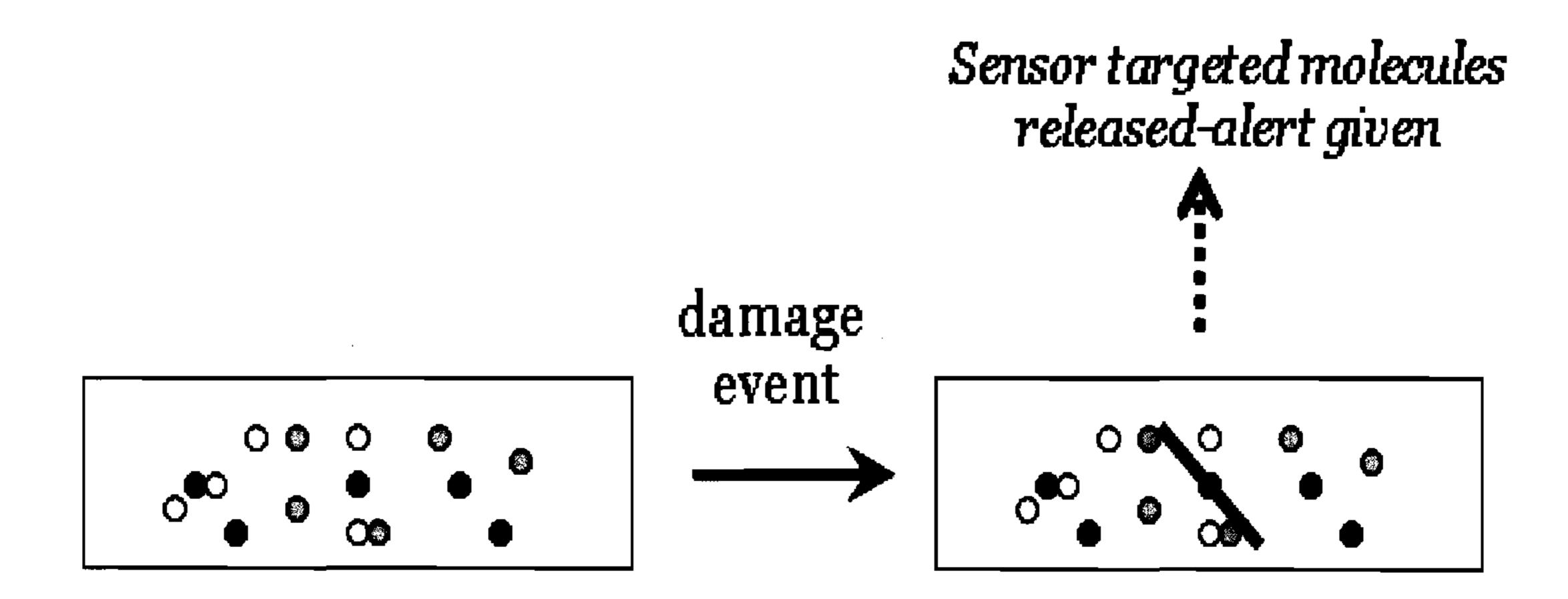
Repair chemicals released to mitigate damage & retain composite strength
