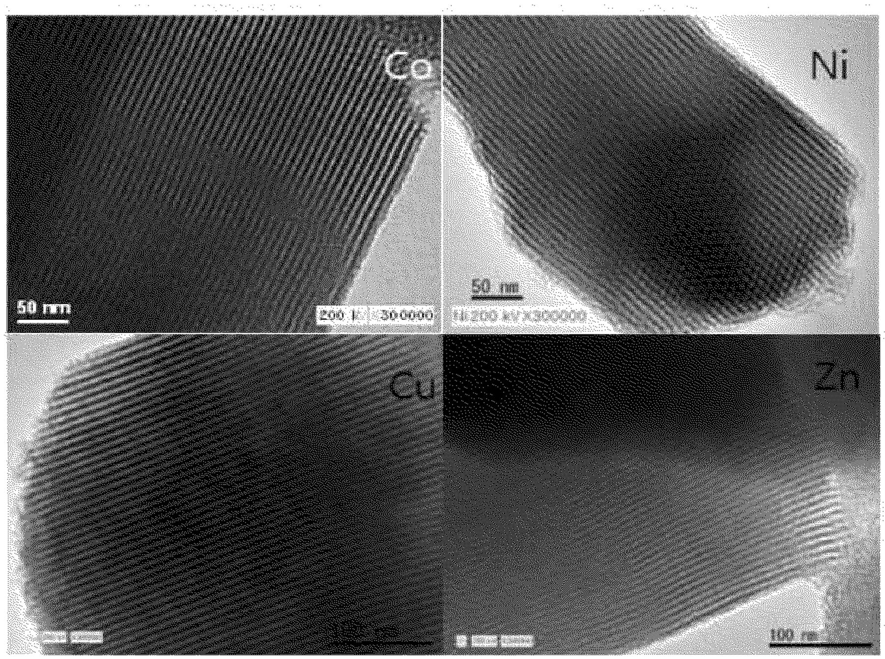
Mesoporous Silica Nanoparticles
