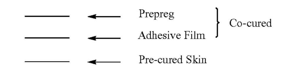
For the secondary bonding studies both adherends are precured. For the co-bonding studies, the cure cycle consists of 2 hours at 350° F. and 85 psi. For the secondary bonding studies, the cure cycle is 90 minutes at 350° F. with 40 psi pressure. After bonding, the specimens are then tested per ASTM D 3165 before and after 2000 hour water soak at 160° F. Lap shear test results are shown in Table 3.
