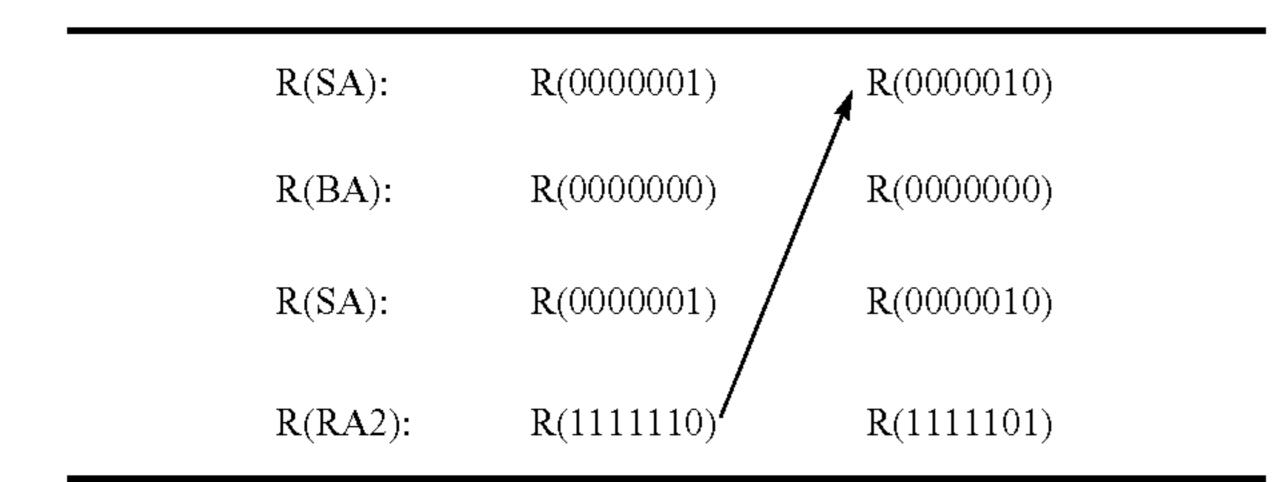
As can be seen, the second refreshing address RA2 (1111110) is responsible for de-selection of the wordlines and bitlines activated by read operations at the shifted address SA (0000001) and the base address BA (0000000). Also, when the hamming distance between the base address BA1 and the base address BA2 is large, say 7, the first refreshing address RA1 may be used.
