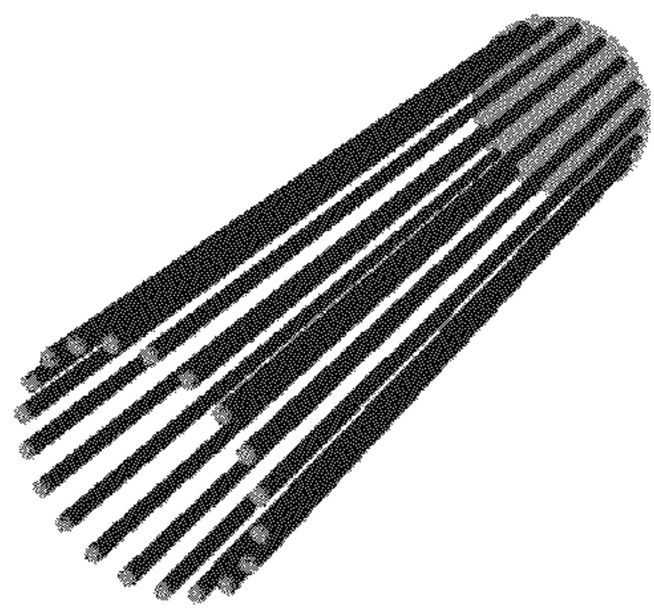
FIG. 7 Thin Walled Tubular Cathode (Prior Art)
