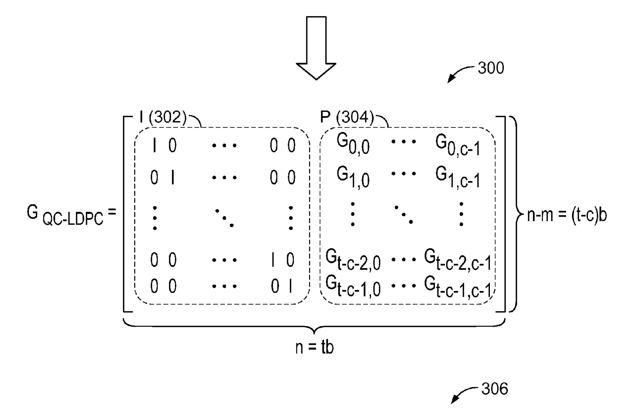
Encoded Data (c) = User Data (u) \* (Generator Matrix )
