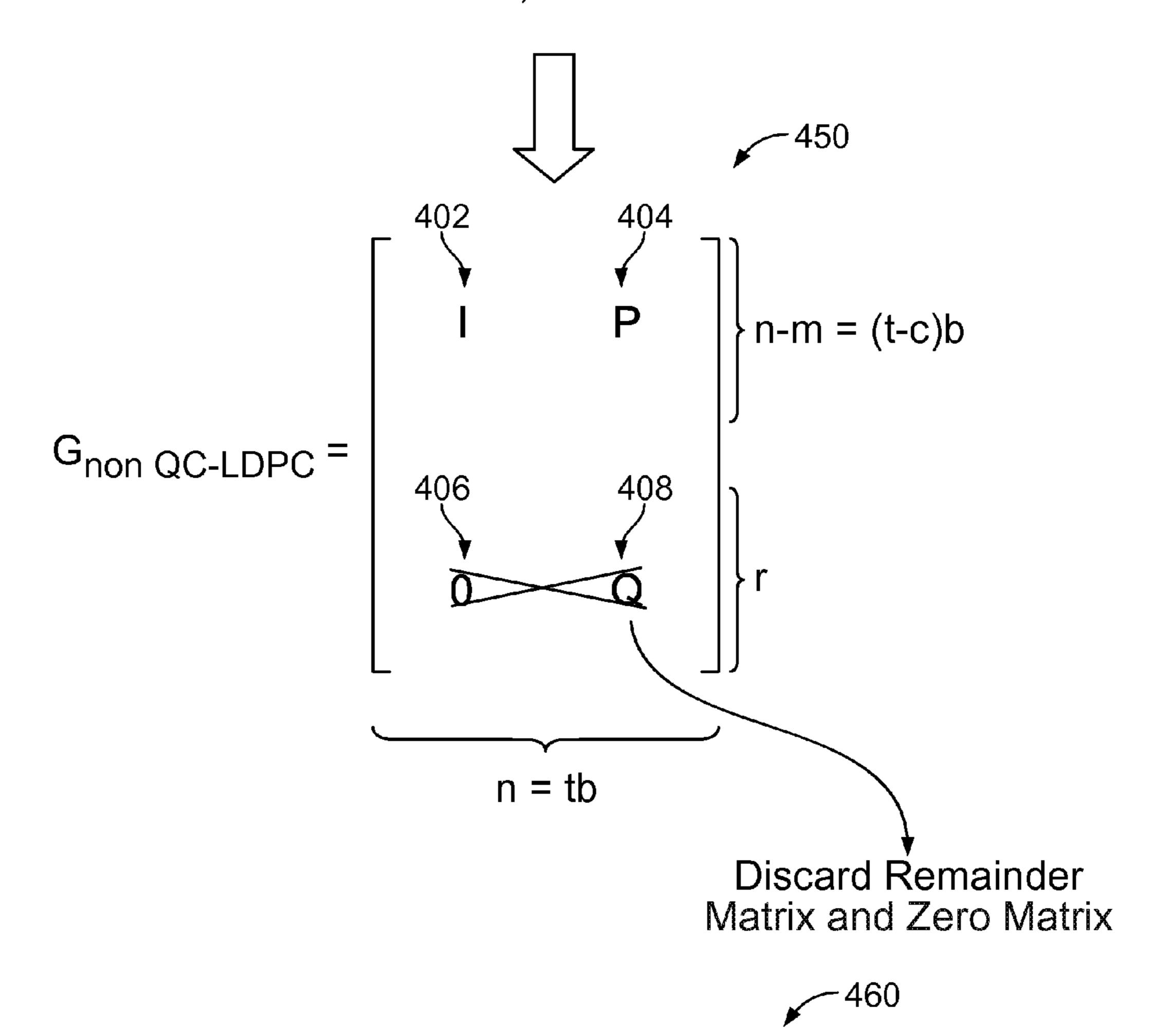
Encoded Data (c) = User Data \* (Generator Matrix with Remainder Matrix and Zero Matrix Discarded)
