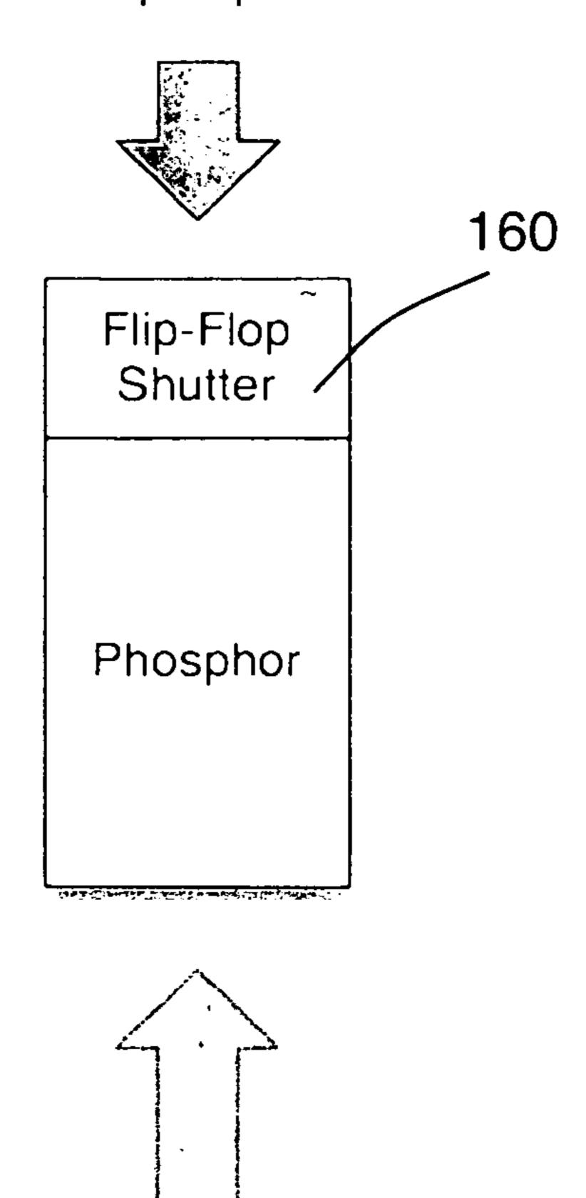
UV Laser beam to charge Phosphor
