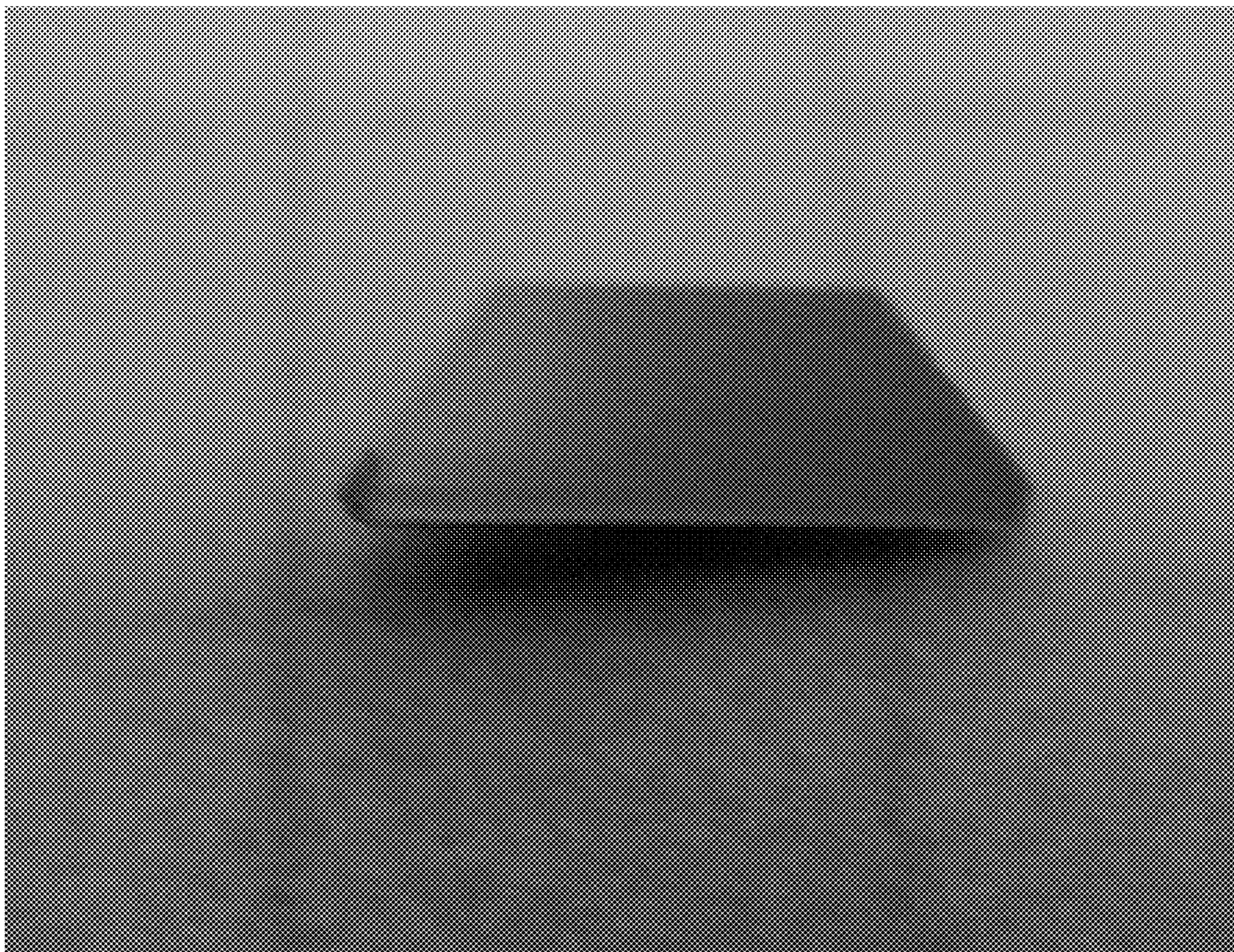
Flat single-crystal; ~7.4mm long; area ~ 0.18cm 2 ; ~75μm thick.
