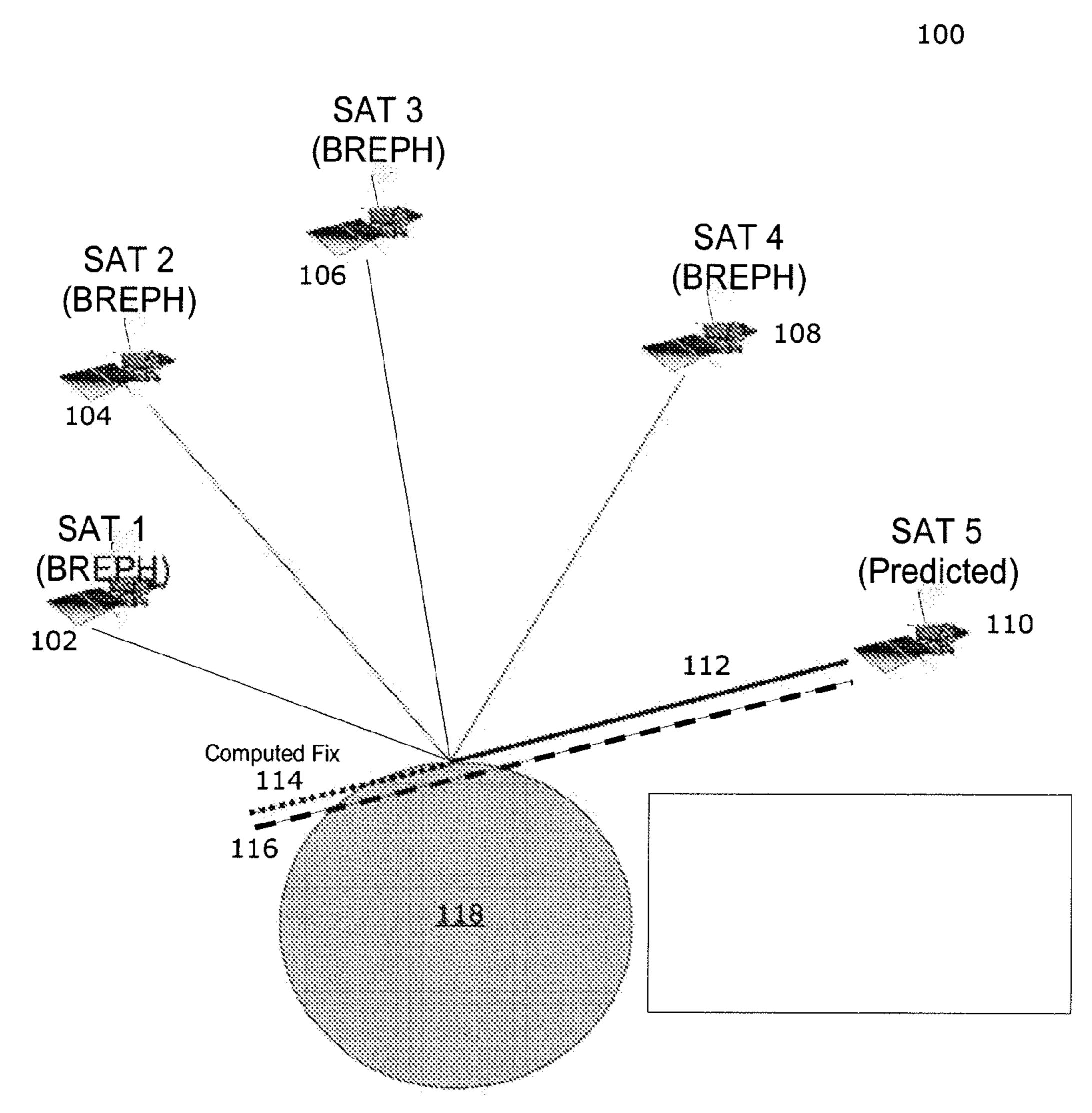
Position is computed using SAT 1 to SAT 4 SAT 5 Clock prediction is corrected
