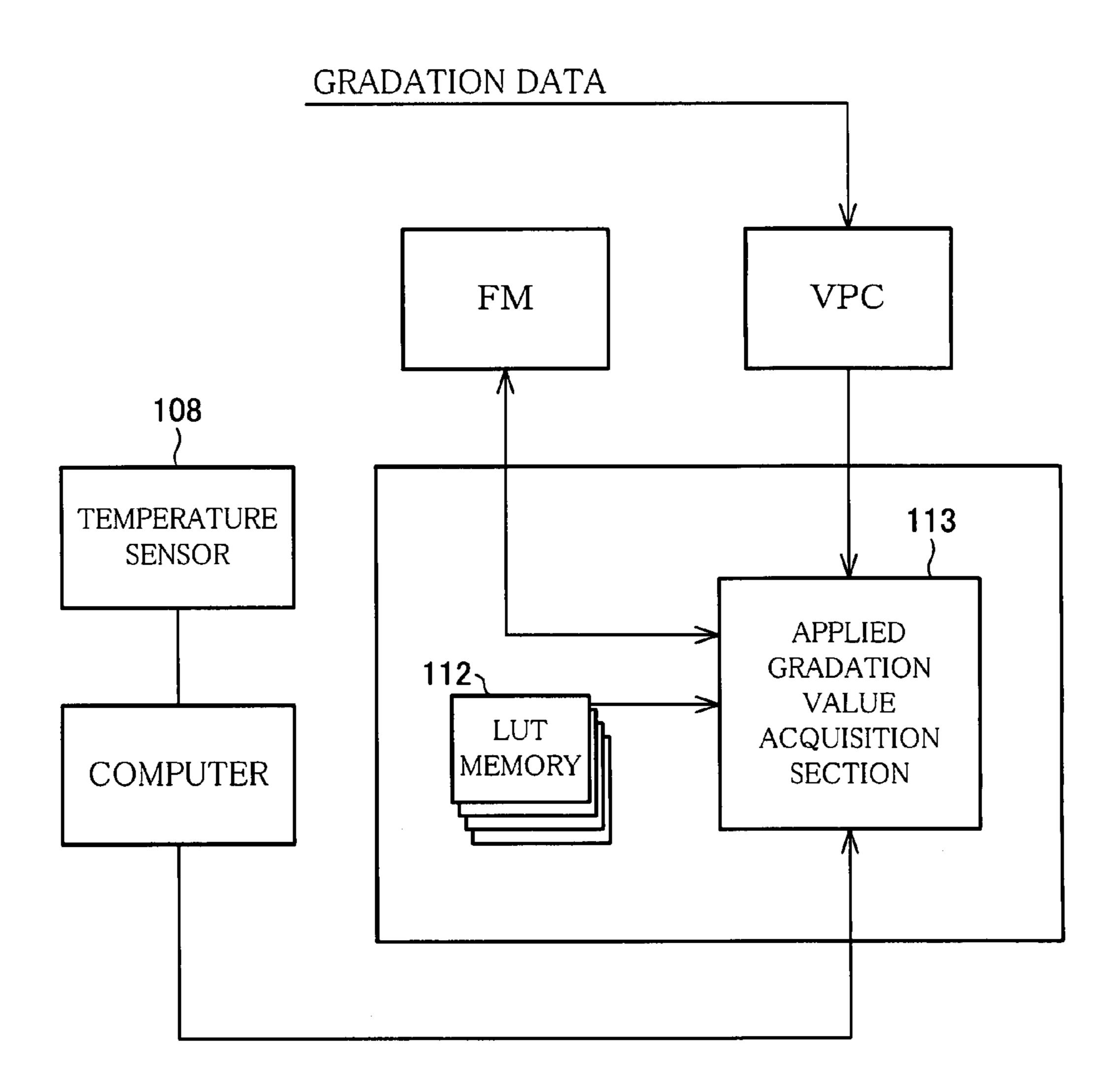
IMAGE DATA PROCESSING DEVICE, LIQUID CRYSTAL DISPLAY APPARATUS INCLUDING SAME, DISPLAY APPARATUS DRIVING DEVICE, DISPLAY APPARATUS DRIVING METHOD, PROGRAM THEREFOR, AND STORAGE MEDIUM
