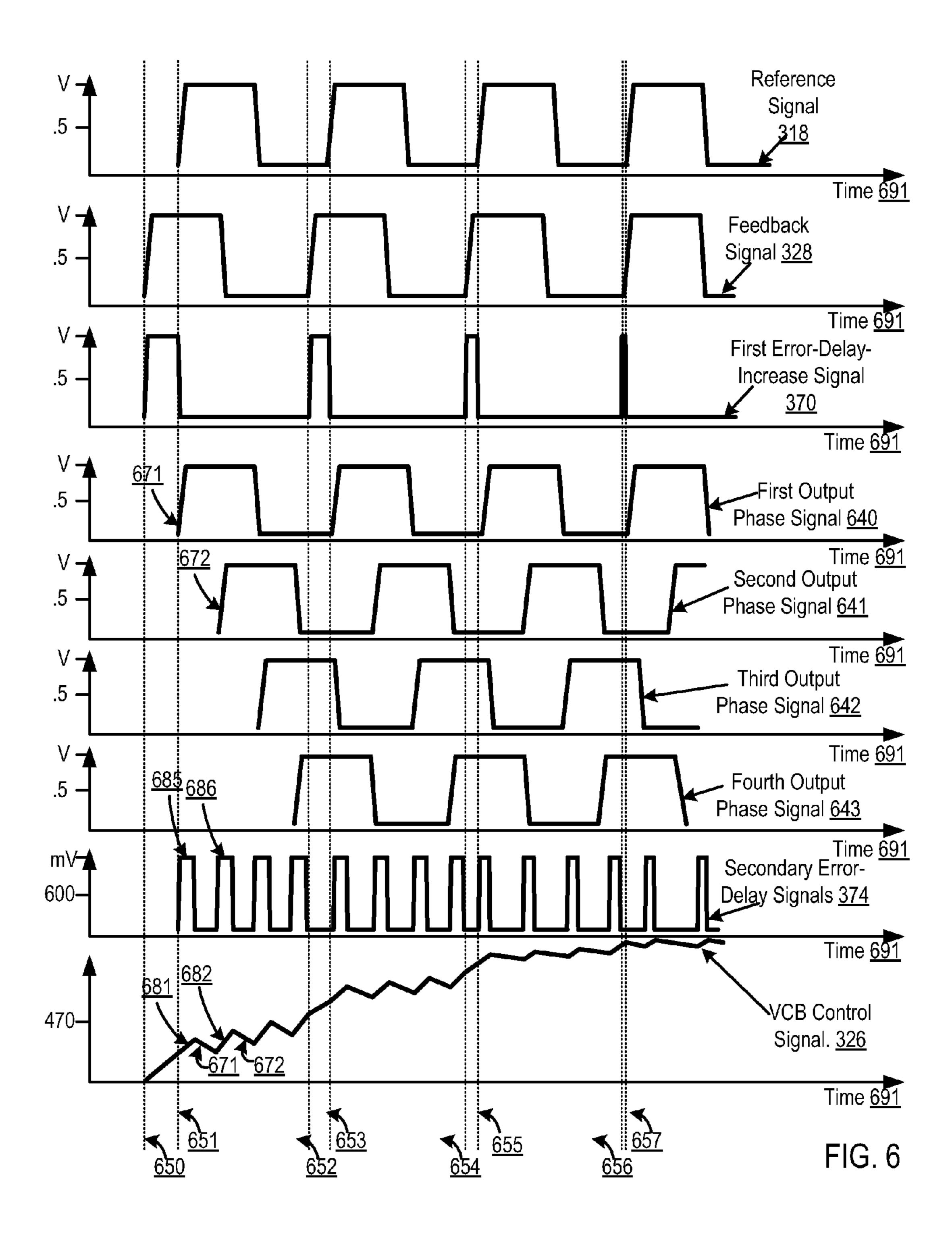
Generate, By A Primary Loop Of A Delay Locked Loop (DLL) Circuit Device, A Feedback Signal Having A Phase That Is Delayed Relative To A Reference Signal, Wherein The Primary Loop Includes A Phase Detector, An Error Controller, And A Voltage Controlled Buffer (VCB) 702
