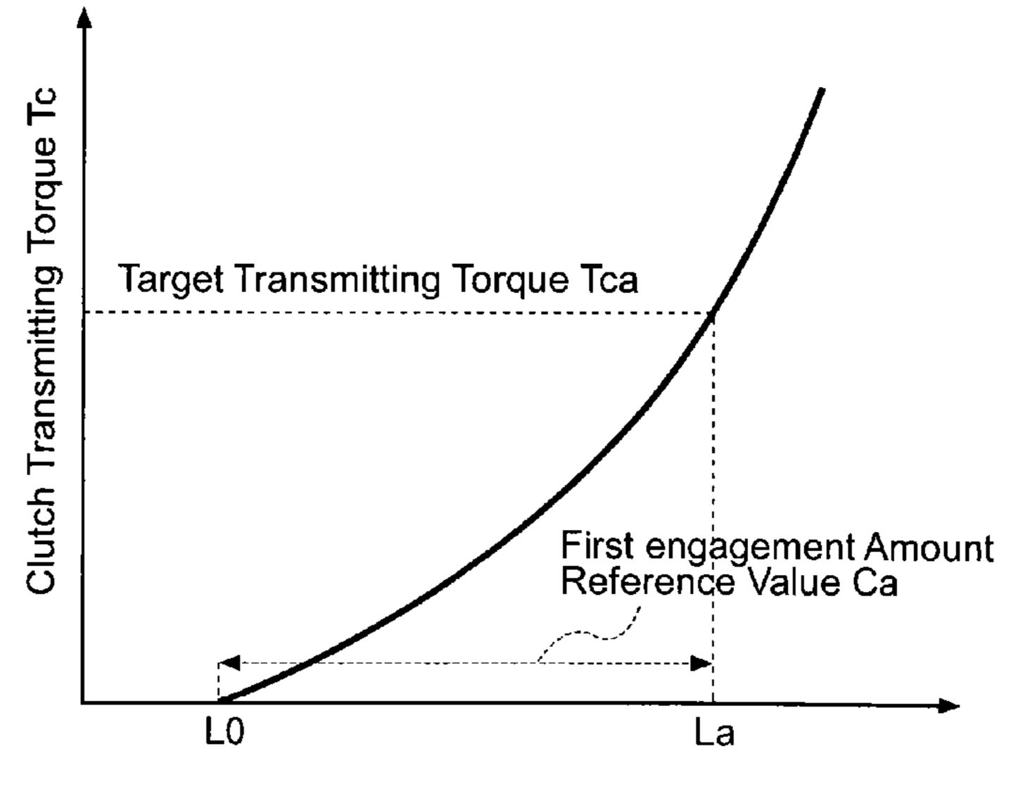
Clutch Actuator Stroke L (Operation Amount)
