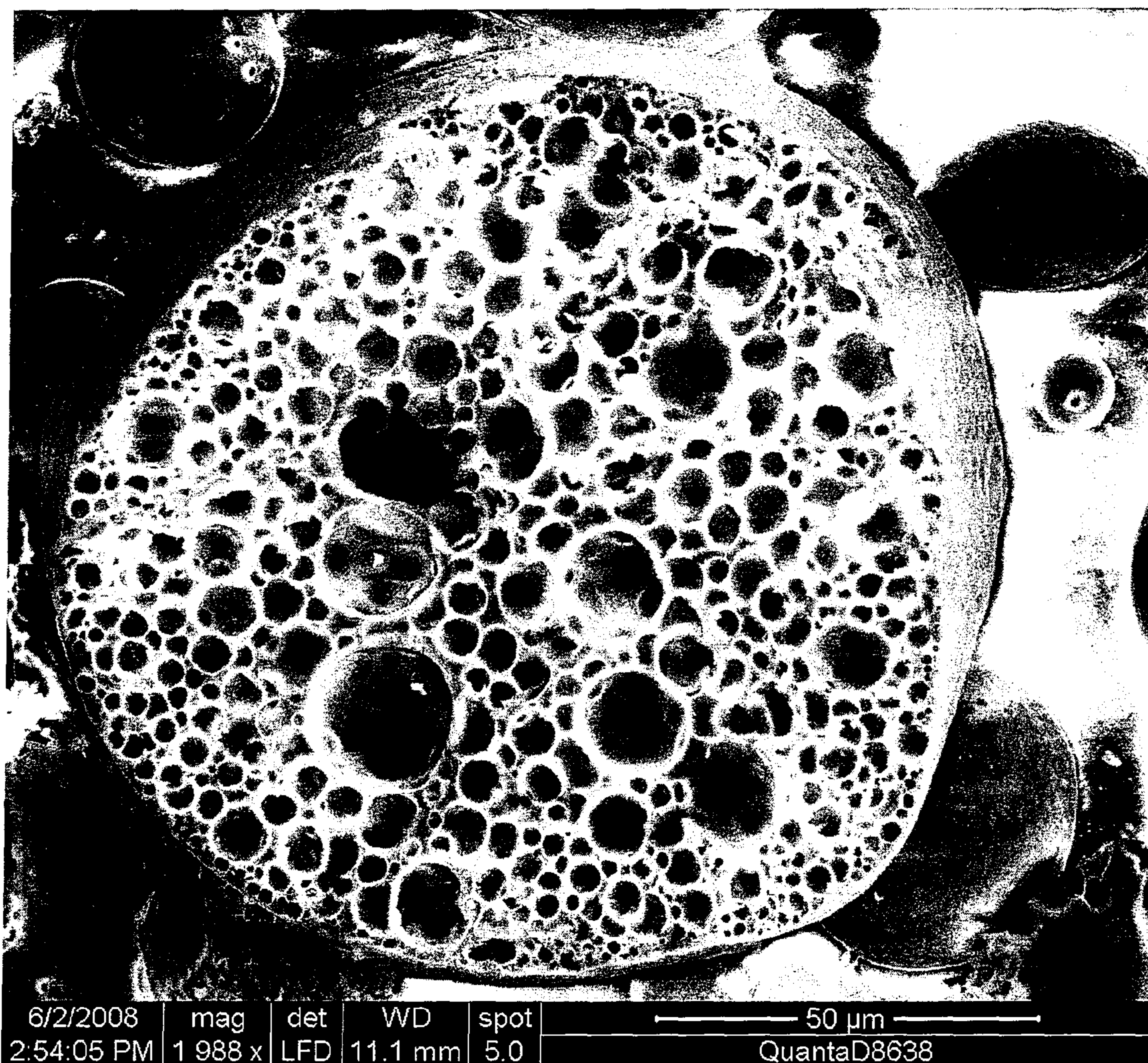
FIG. 4C: Particle Cross-Section at 1988x Magnification
