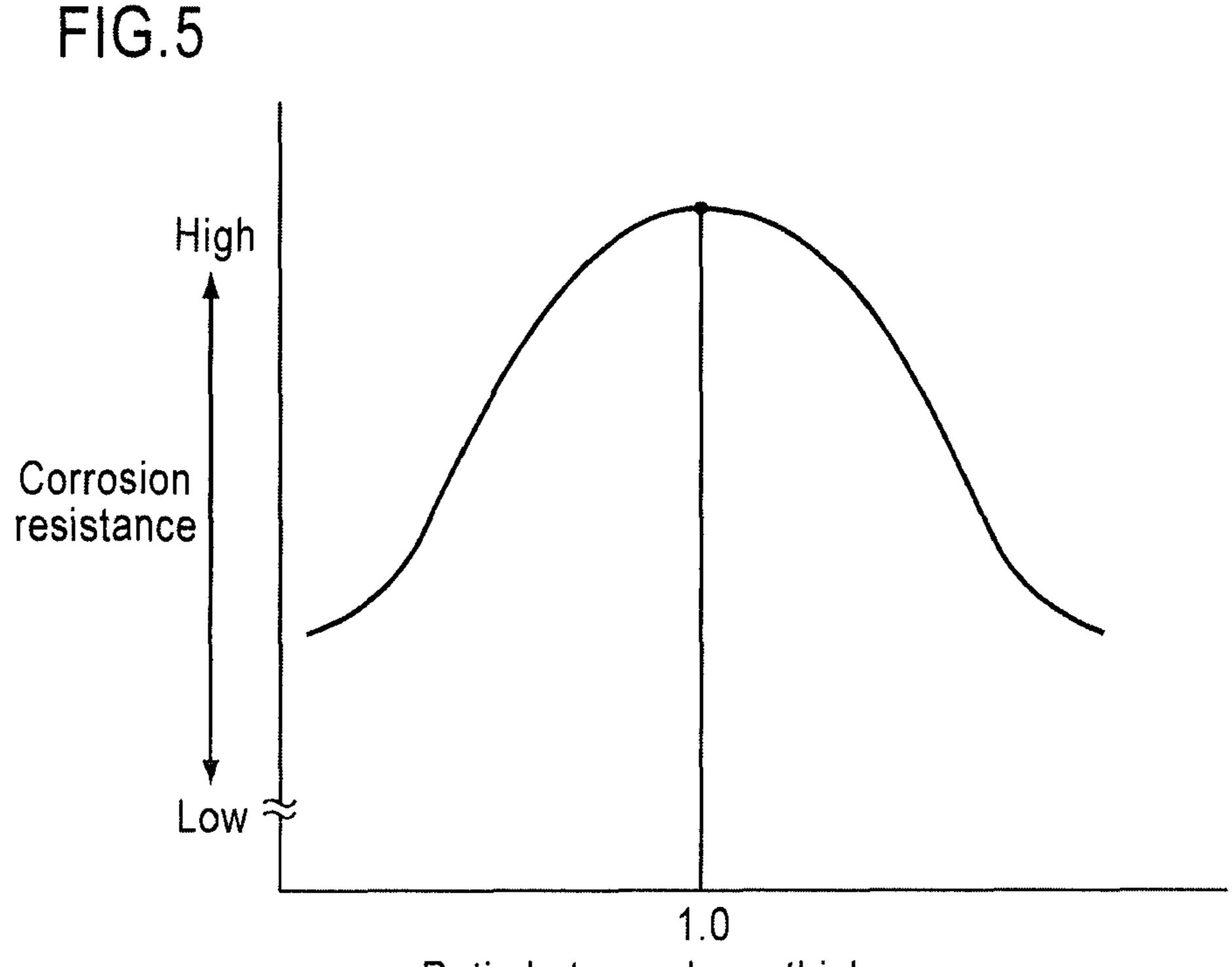
Ratio between layer thicknesses (ratio of thickness of semibright nickel plating layer to thickness of bright nickel plating layer)
