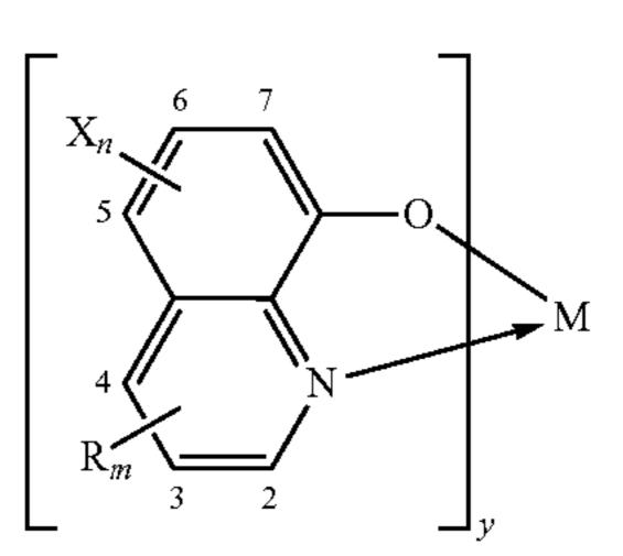
wherein M represents a divalent or a trivalent metal; each of X and R may independently be chosen from the group consisting of halogen, cyano, carboalkoxy, alkyl, alkoxy, aryl, hetaryl, carboxy, hydroxy, sulfo and phospho substituents; n and m independently represent an integer from 0-3; and the number of ligands y is 2 or 3; with the proviso that n+m is an integer from 1 to 6, and at least one of X and R comprises a solubilizing group capable of imparting water solubility to the complex.
