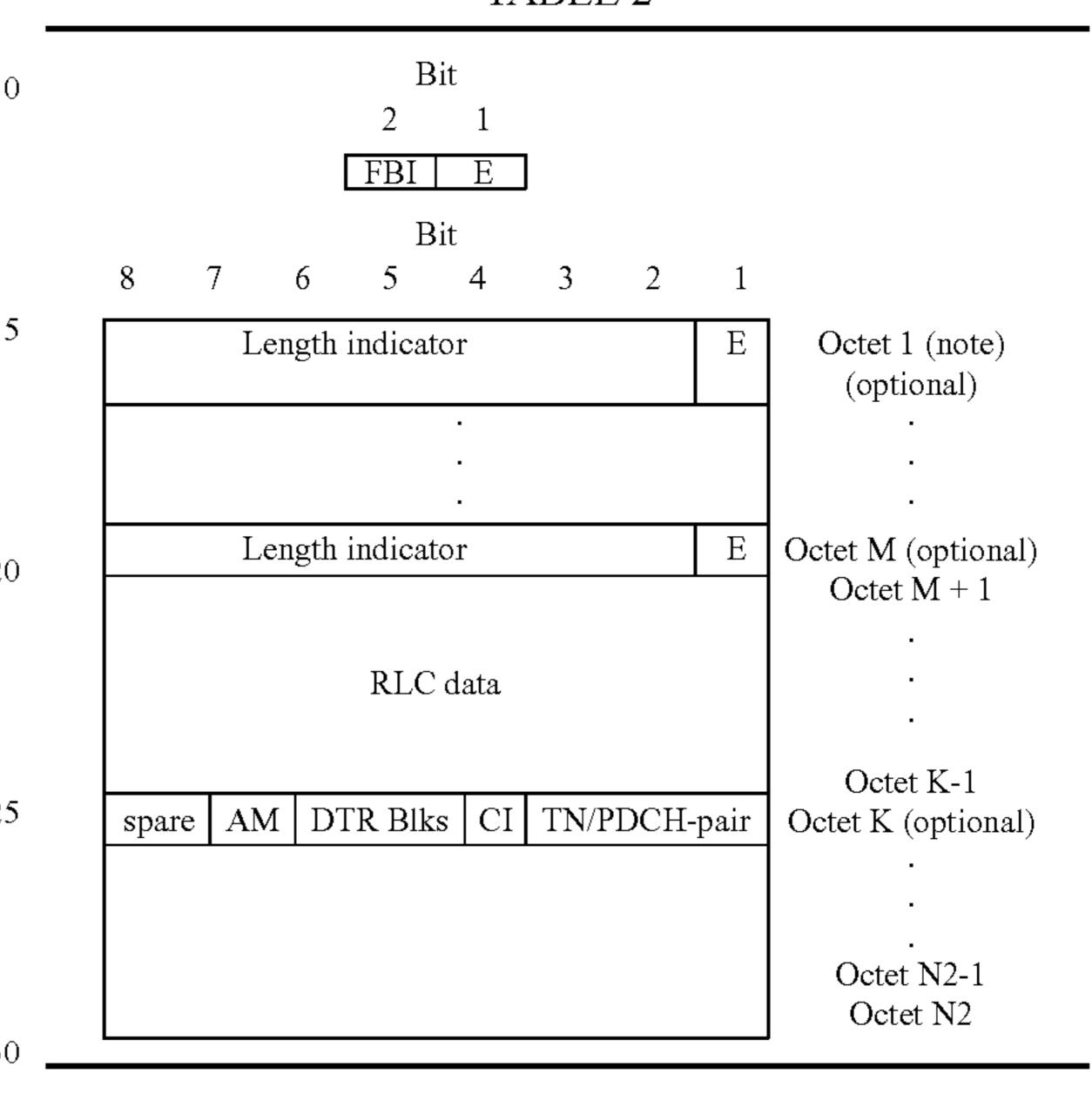
The AM field indicates the DTR activation procedure the mobile station shall follow during a downlink TBF. Accordingly, the radio blocks monitored in DTR mode include:
