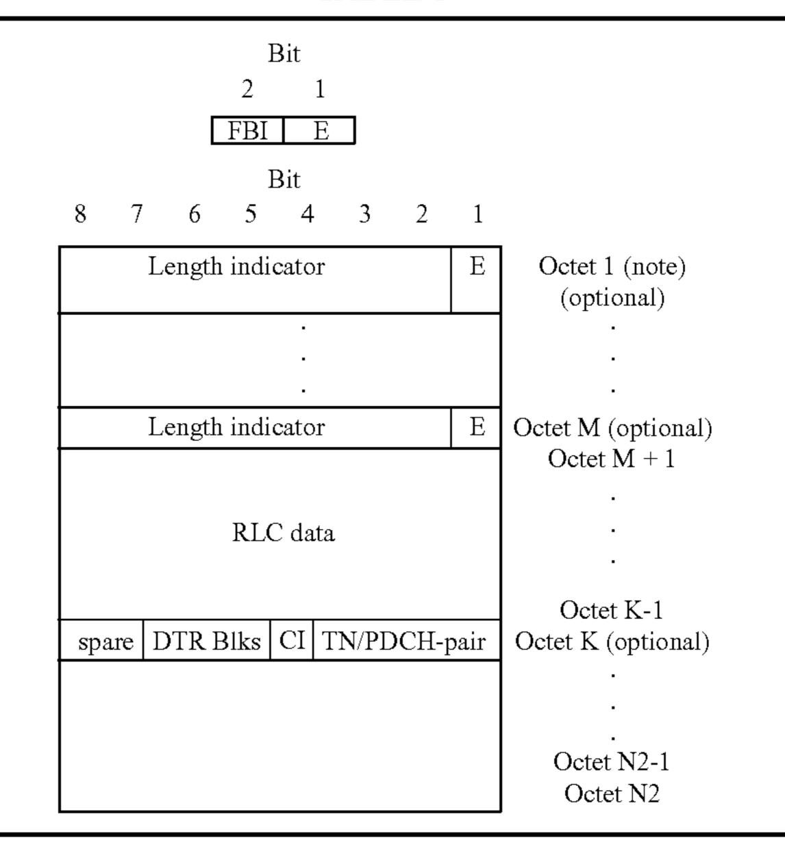
Referring to Table 1, the carrier ID (CI) field contains a identification of the carrier that may be encoded as DTR\_CI
