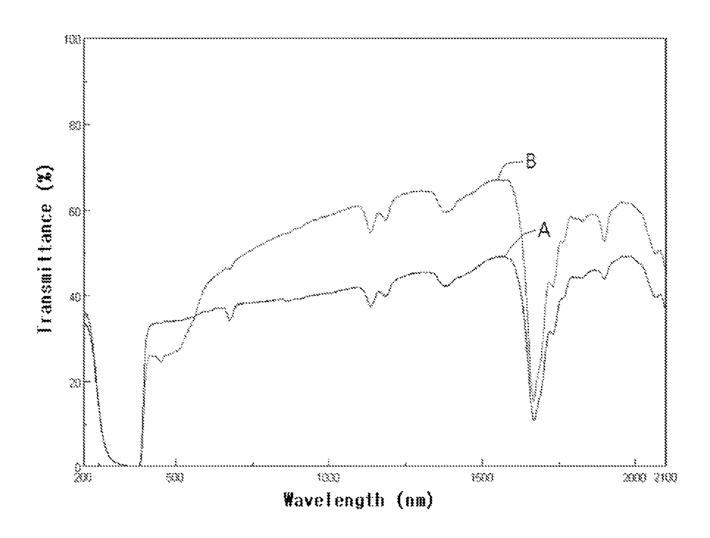
A: Graph showing infrared transmittance of multifunctional optical sheet having light shielding property
