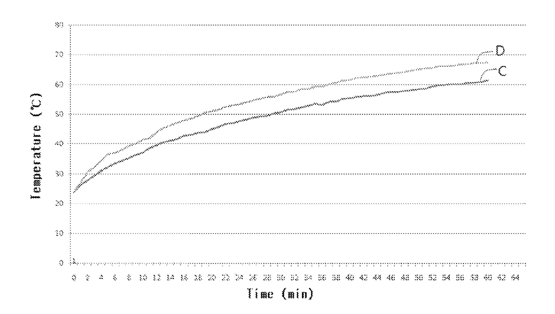
C: Graph showing thermal insulating effect of multifunctional optical sheet having light shielding property
