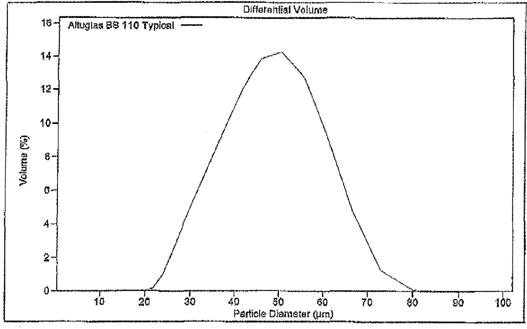
Altuglas BS 110 Typical Volume Statistics (Arithmetic) Calculations from 0.375 µm to 2,000 µm 100% Volume: 11.08 µm 45.88 µm \$.D.; Mean: C.V.: 24.1% Median: 45.62 µm D(3,2): 43.10 µm Mode: 50.22 µm dşo: 61.06 µm <10% <25% <75% <90% <50% 37.44 µm 45.62 µm 63.92 µm 61.06 µm 31.15 µm
