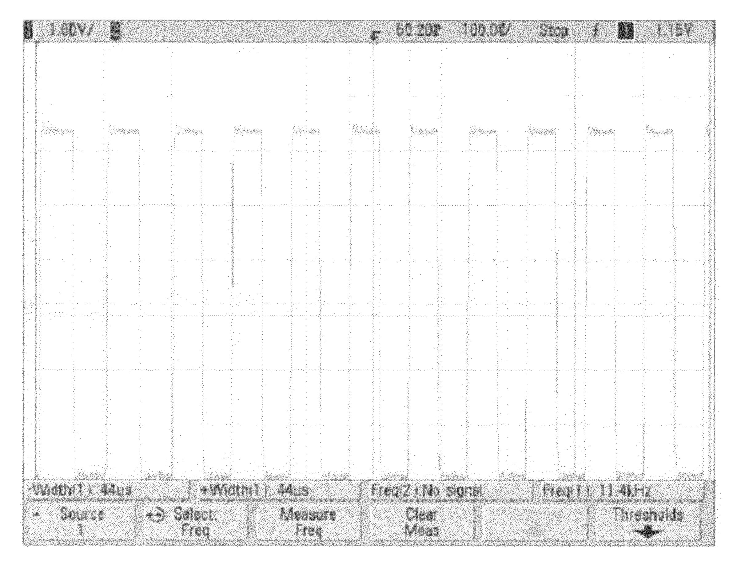
Vavetorm after 50.2 msec has elapsed Frequency increase to 11.4KHz Waveforms from later in the event have not been included
