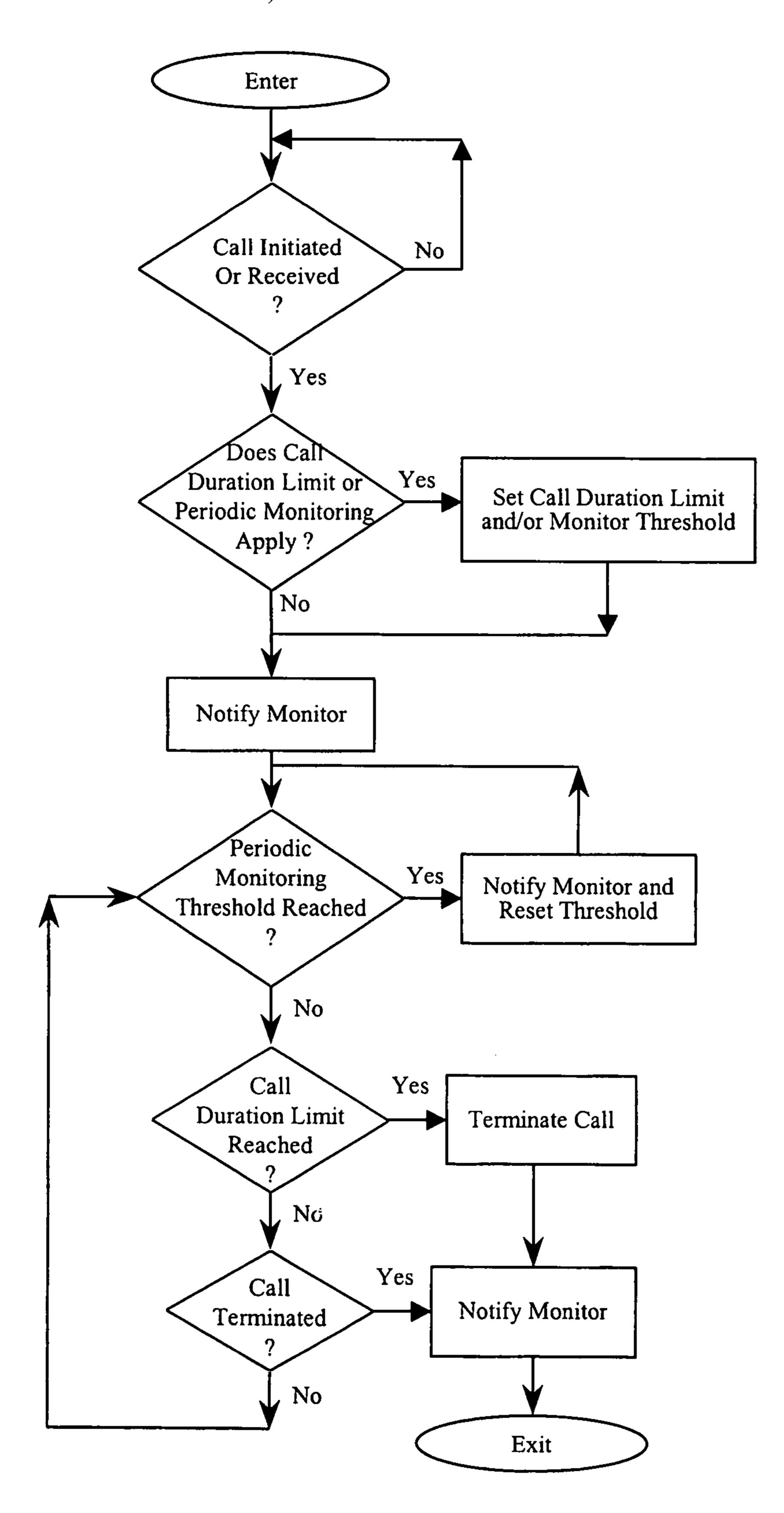
Figure 3 – Monitor Notification Flow
