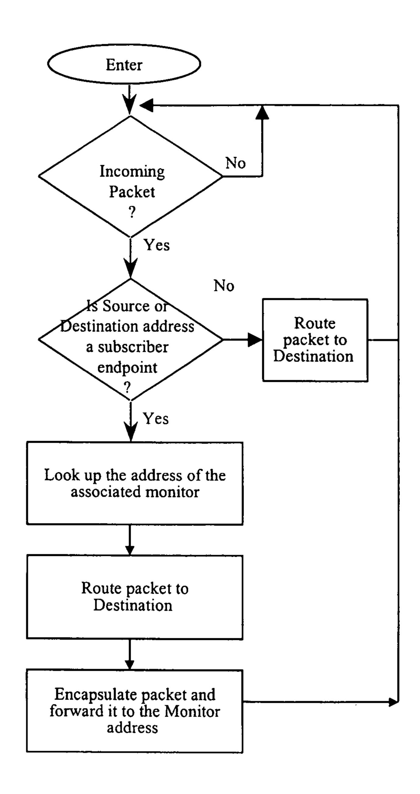
Figure 6 – Gateway Flow Logic
