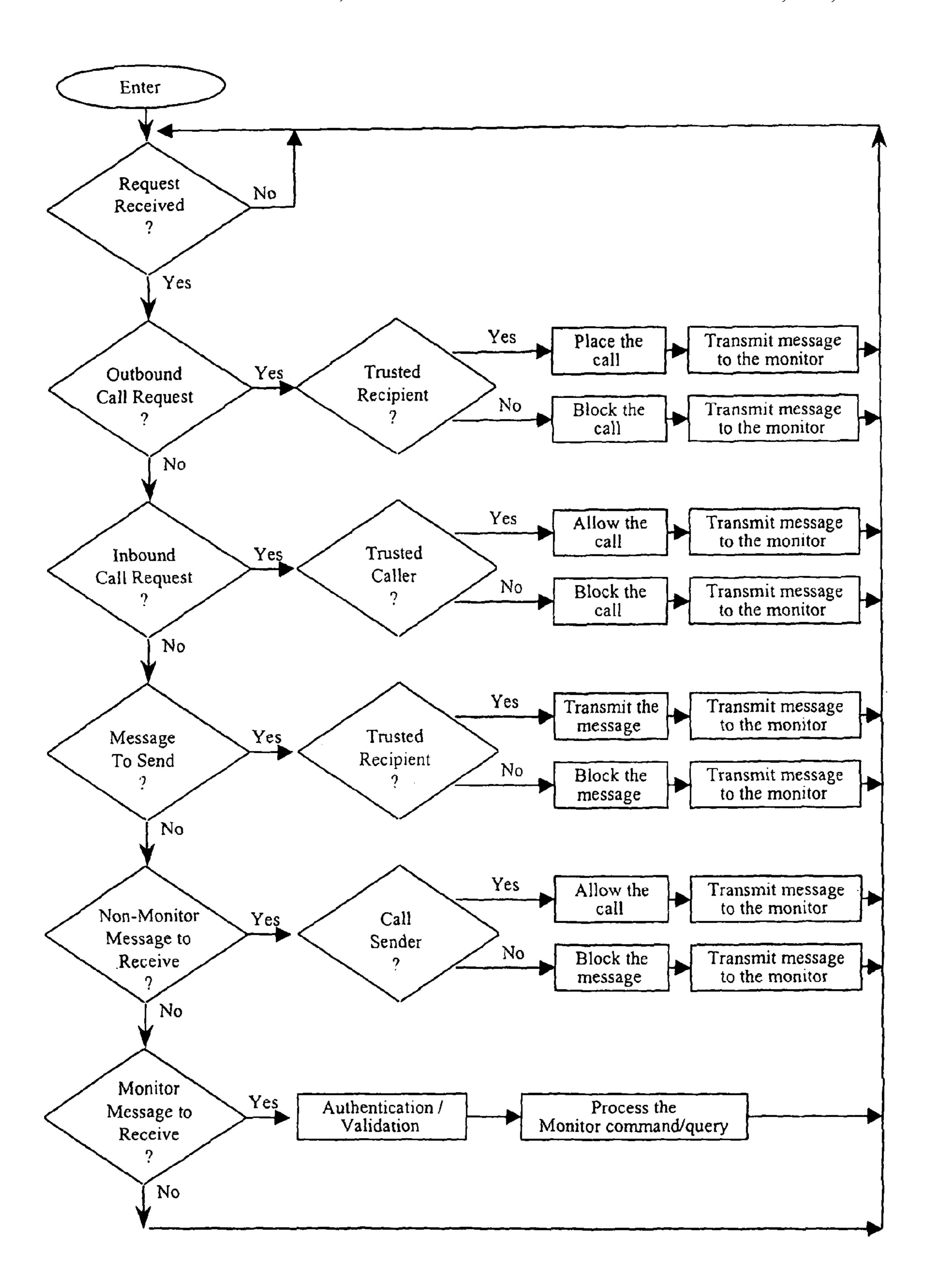
Figure 2 –Flow Logic
