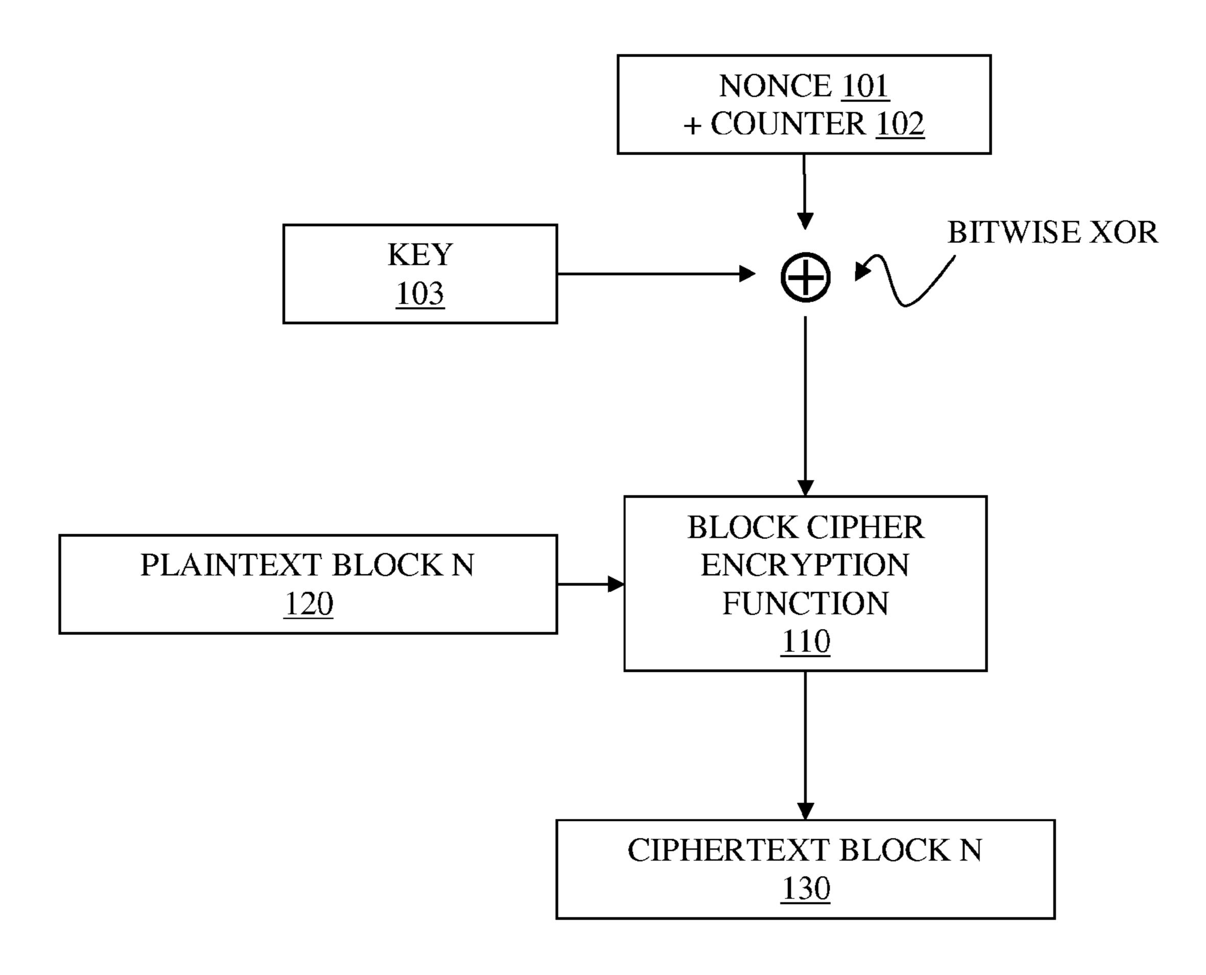
N-TH CIPHERTEXT BLOCK  $c_n = E_{(k \oplus n)}(p_n)$
