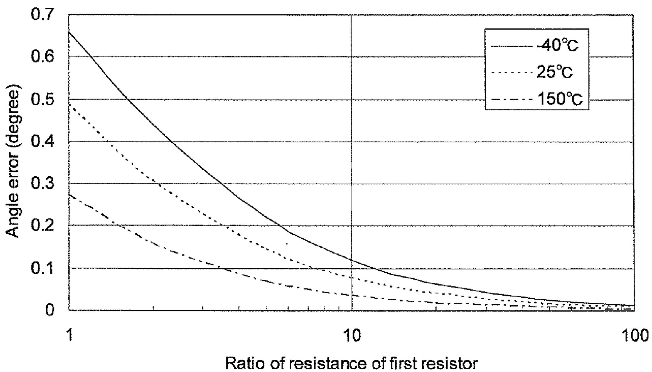
to minimum resistance of first resistor to minimum resistance of bridge circuit (R21/Rmin)
