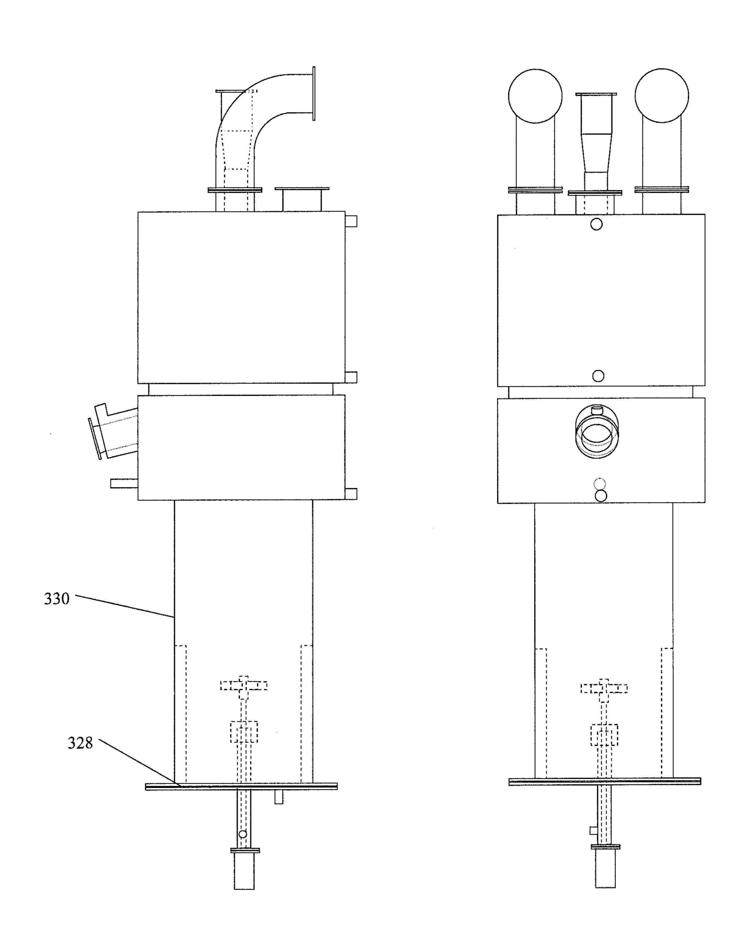
FIGURE 4: JET SCRUBBER AND WAX SEPARATOR
