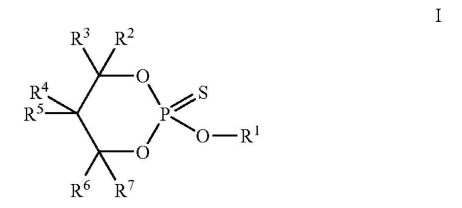
where R<sup>1</sup>, R<sup>2</sup>, R<sup>3</sup>, R<sup>4</sup>, R<sup>5</sup>, R<sup>6</sup>, and R<sup>7</sup> are as defined herein. Such a compound may exhibit improved antiwear performance and thermal stability in lubricating compositions.
