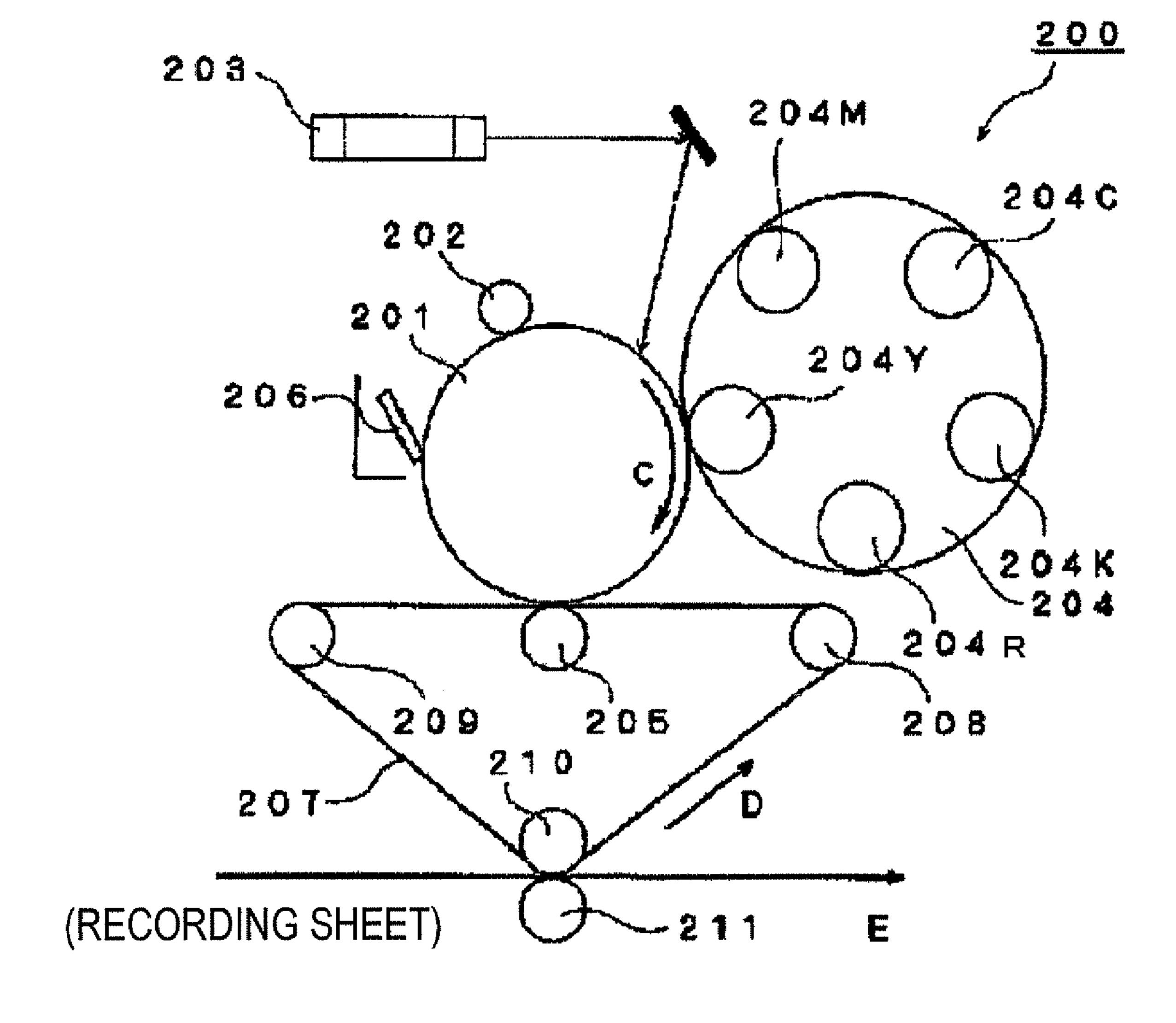
RED TONER FOR ELECTROSTATIC IMAGE DEVELOPMENT, DEVELOPER FOR ELECTROSTATIC IMAGE DEVELOPMENT, TONER SET FOR ELECTROSTATIC IMAGE DEVELOPMENT, DEVELOPER SET FOR ELECTROSTATIC IMAGE DEVELOPMENT AND IMAGE FORMING APPARATUS
