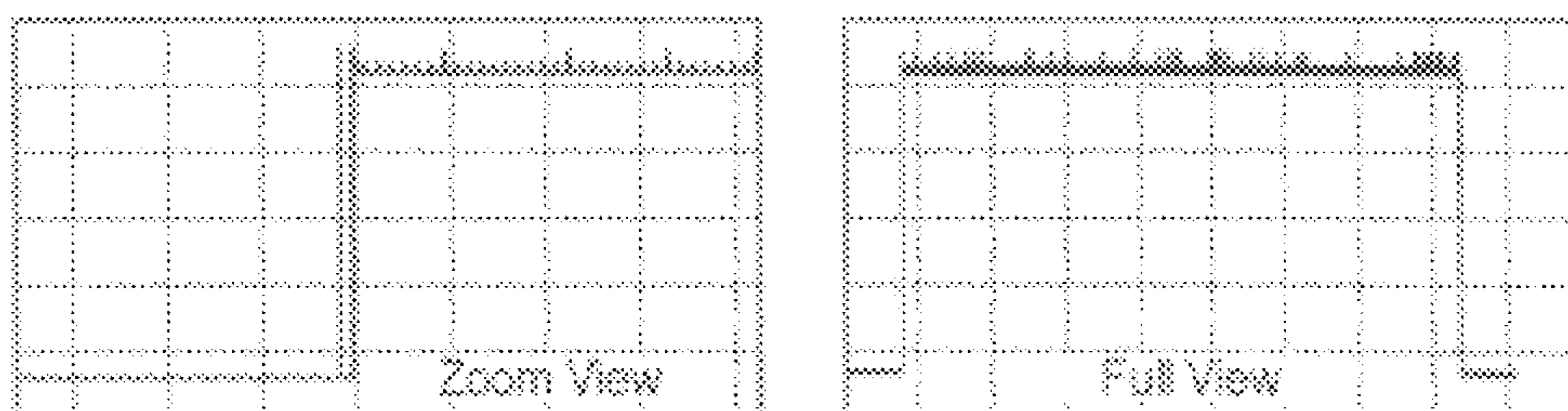
11 Notched Carriers at Transmitter Output, Left Hand Edge of OFDM Spectrum
