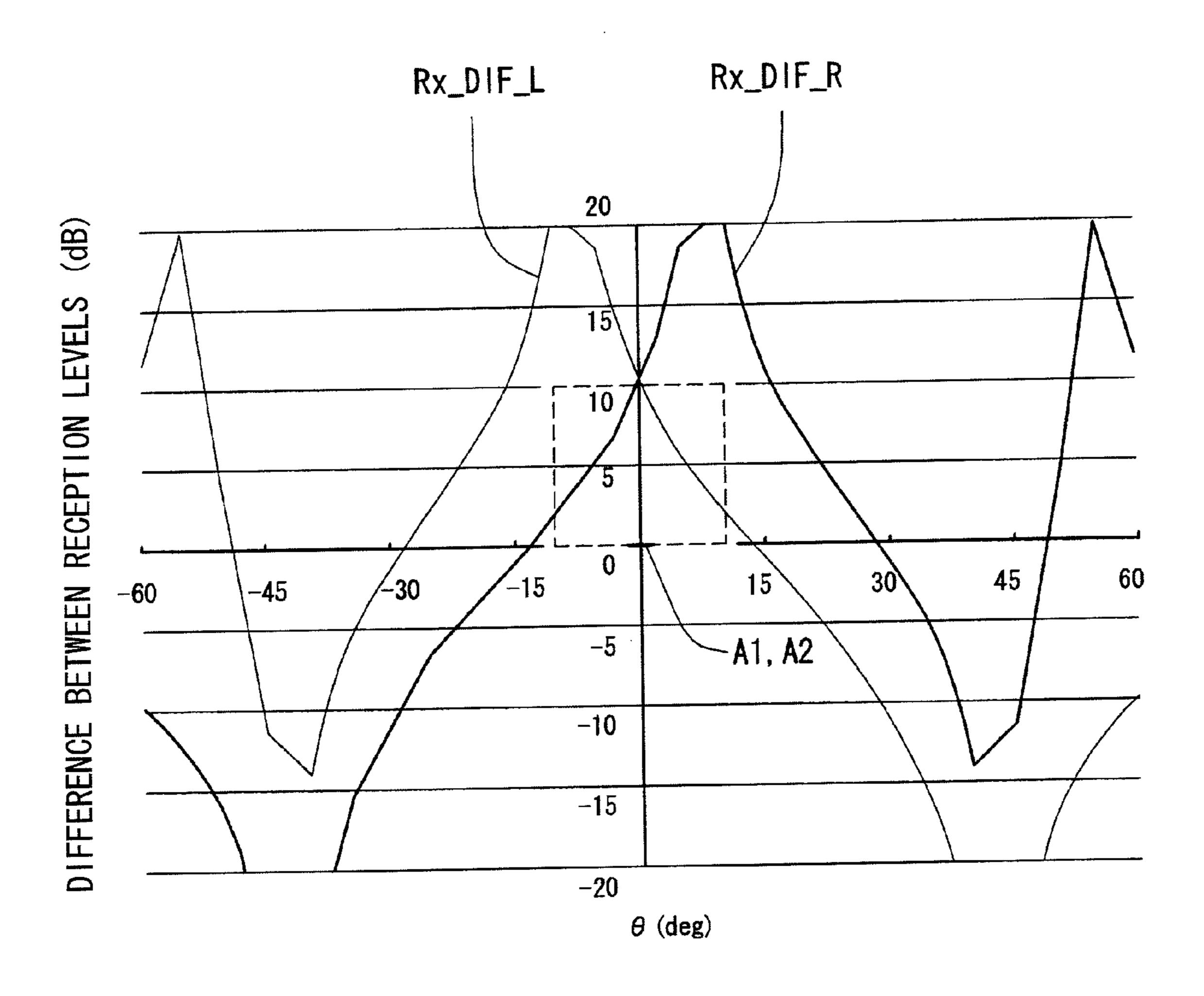
A1, A2···THRESHOLD Rx\_DIF\_L---LEFTWARD RECEPTION LEVEL RATIO Rx\_DIF\_R---RIGHTWARD RECEPTION LEVEL RATIO
