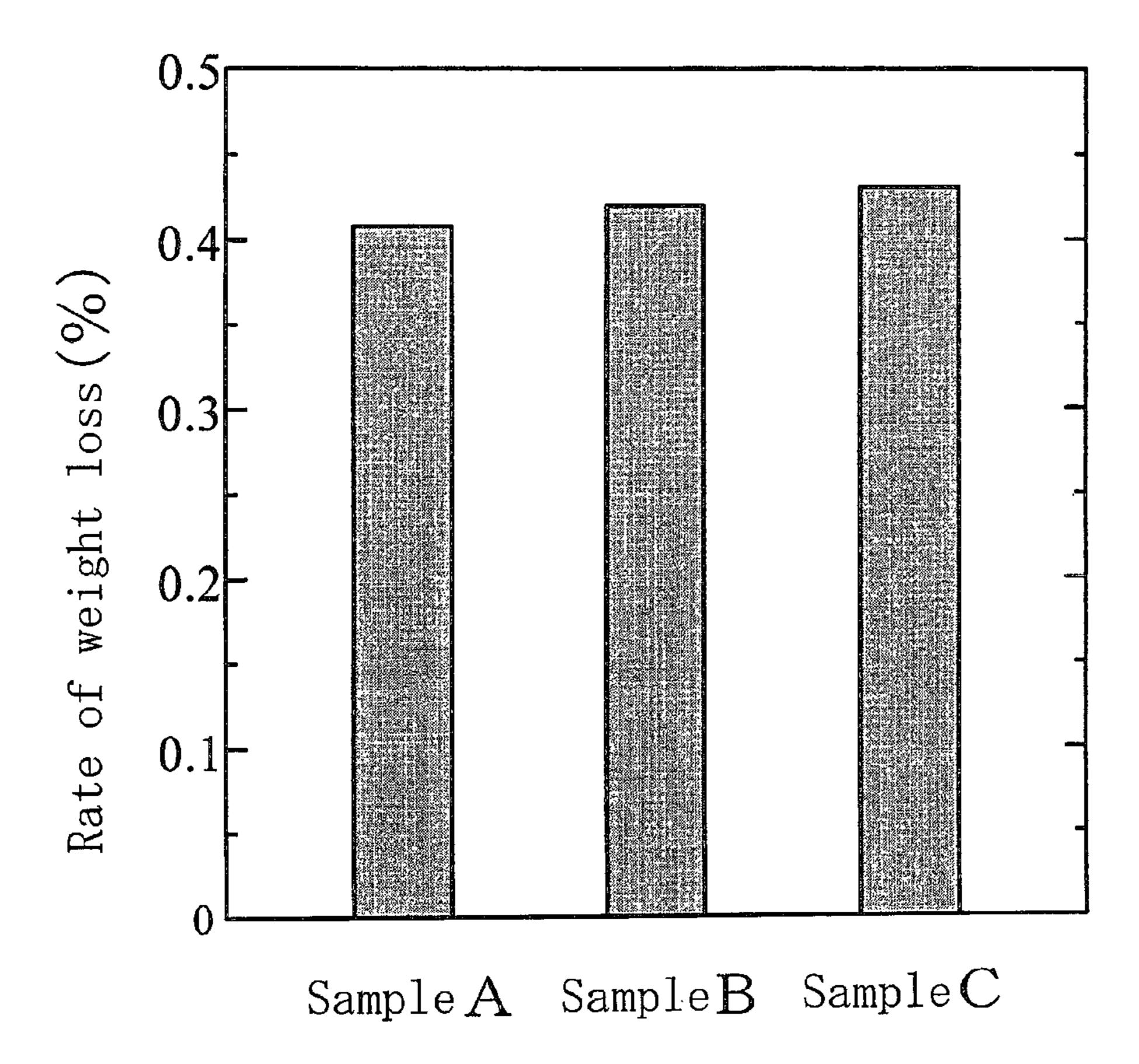
Sample A: Conventional free-cutting alloy (containing Sn-Bi)-T3 Sample B: Alloy according to this invention (containing 1.0%Bi)-T3 Sample C: Alloy according to this invention (containing 1.5%Bi)-T3
