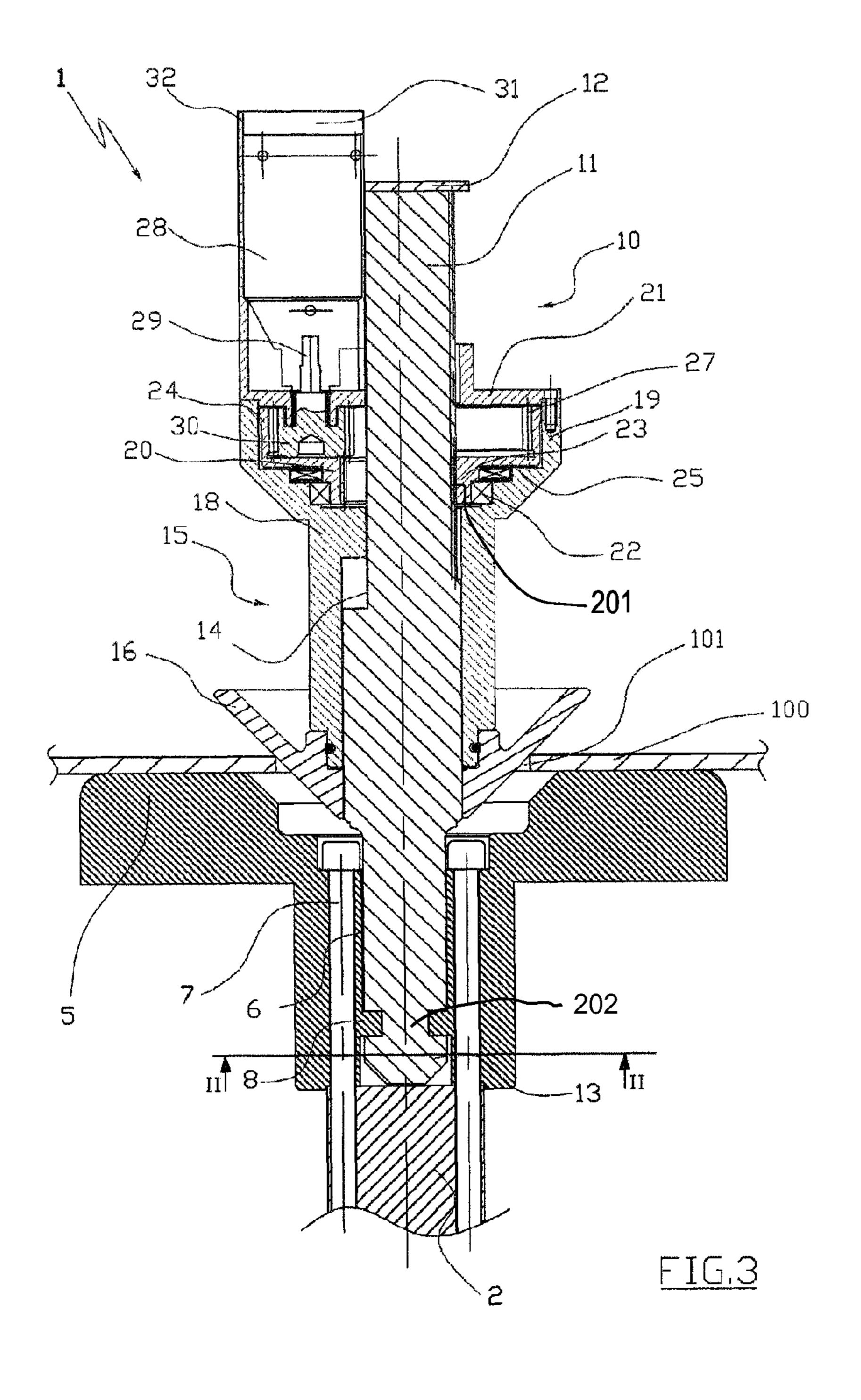
The invention relates to a self-centring device for blocking a wheel rim in a working position on a tyre-mounting machine, with the aim of fitting or removing a tyre from the
