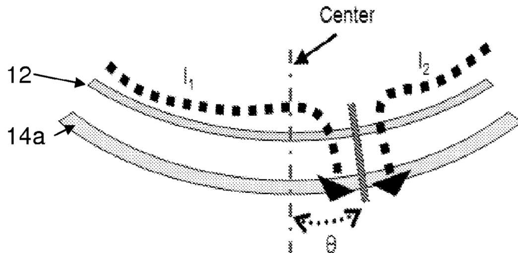
The angle  $\theta$  is derived from the difference in the resistances (and therefore currents) on each side of the connection.
