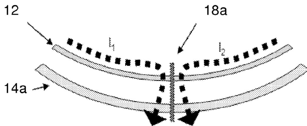
If the contact is exactly centered,  $I_1 = I_2$ . (Assuming  $V_1 = V_2$ )
