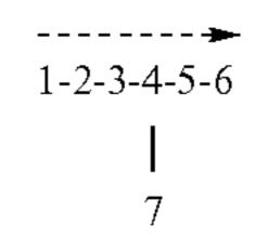
With the data flow from node 1 to node 6, step S2 says start with an empty schedule and step S4 says assign the source node (node 1) a transmit time in the first slot.
