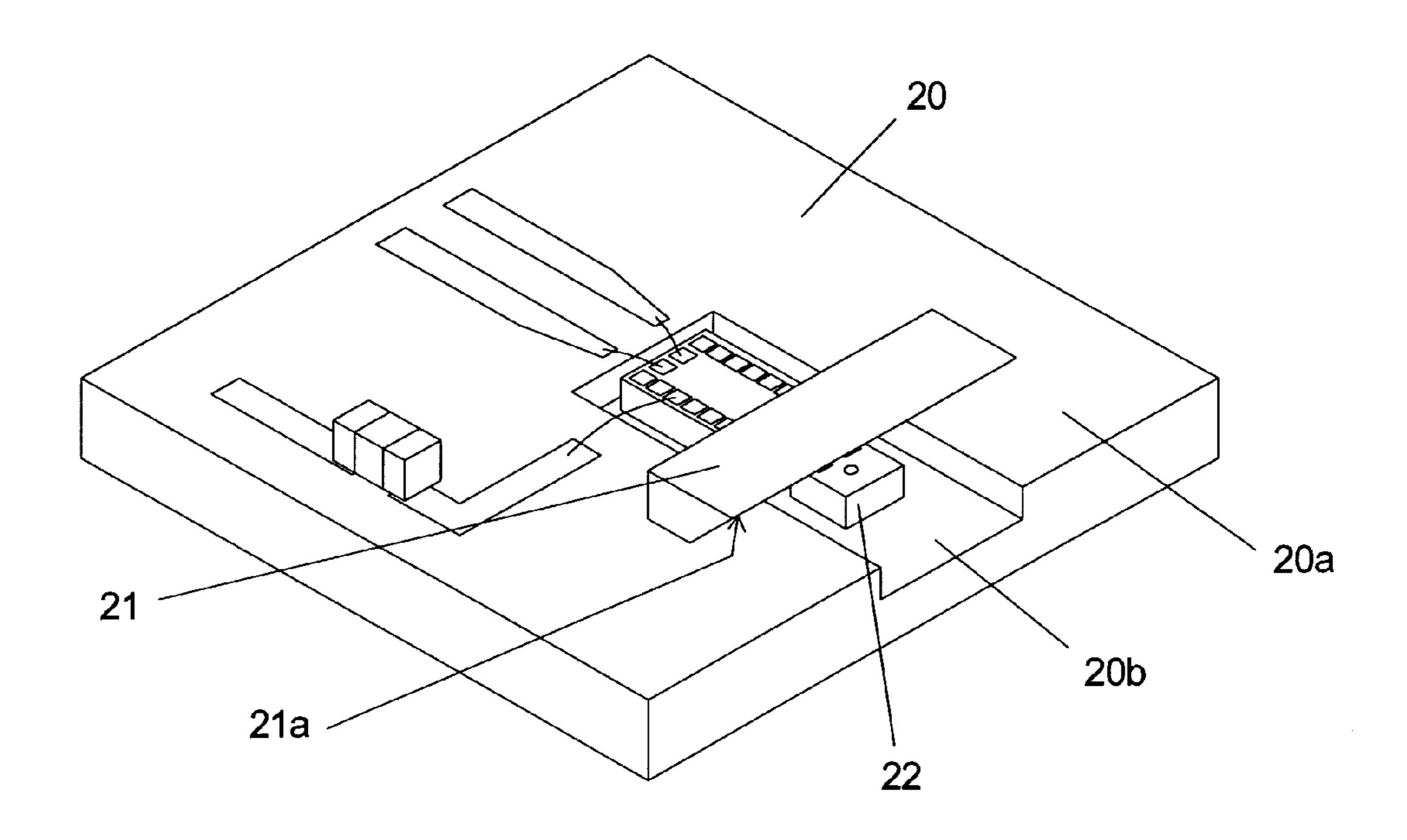
Figure 5: Front view of embodiment with a micro-mirror having a structured bottom side
