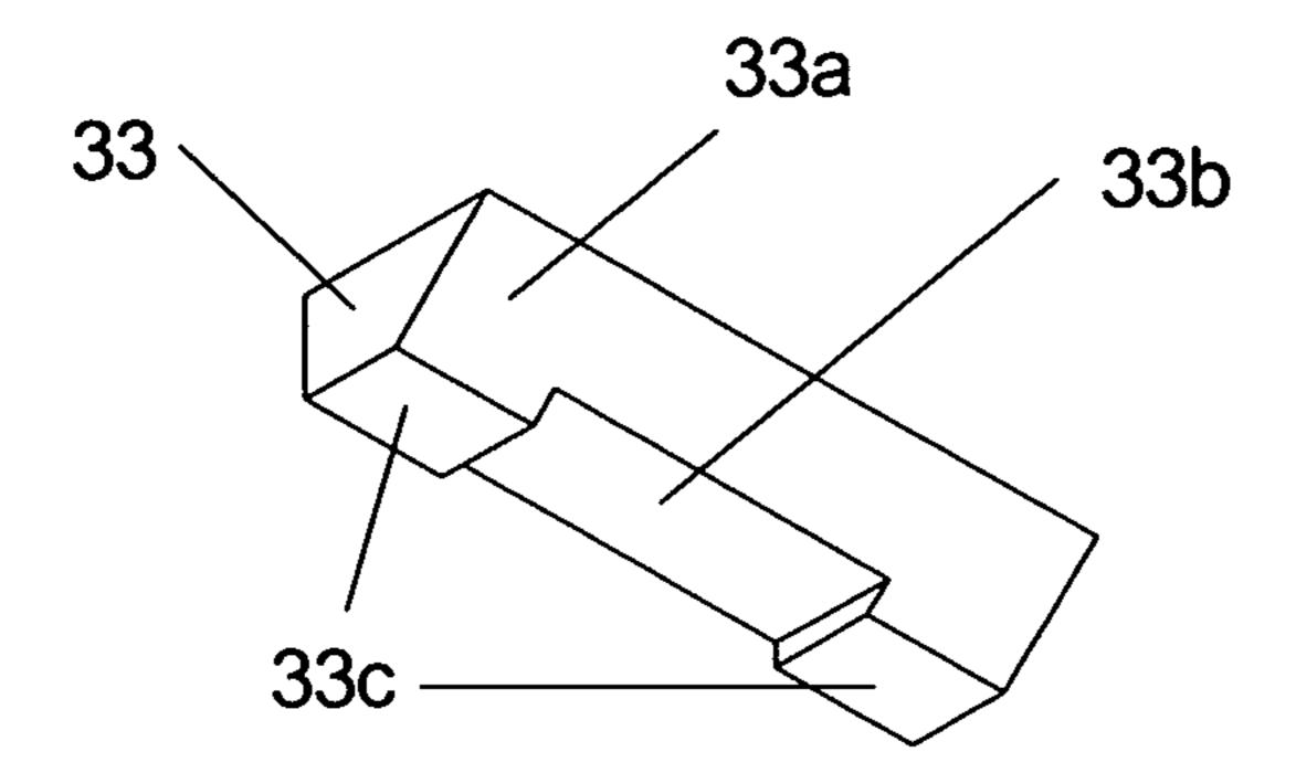
Figure 7: Assembly with mounting plate with areas of different height on the top surface
