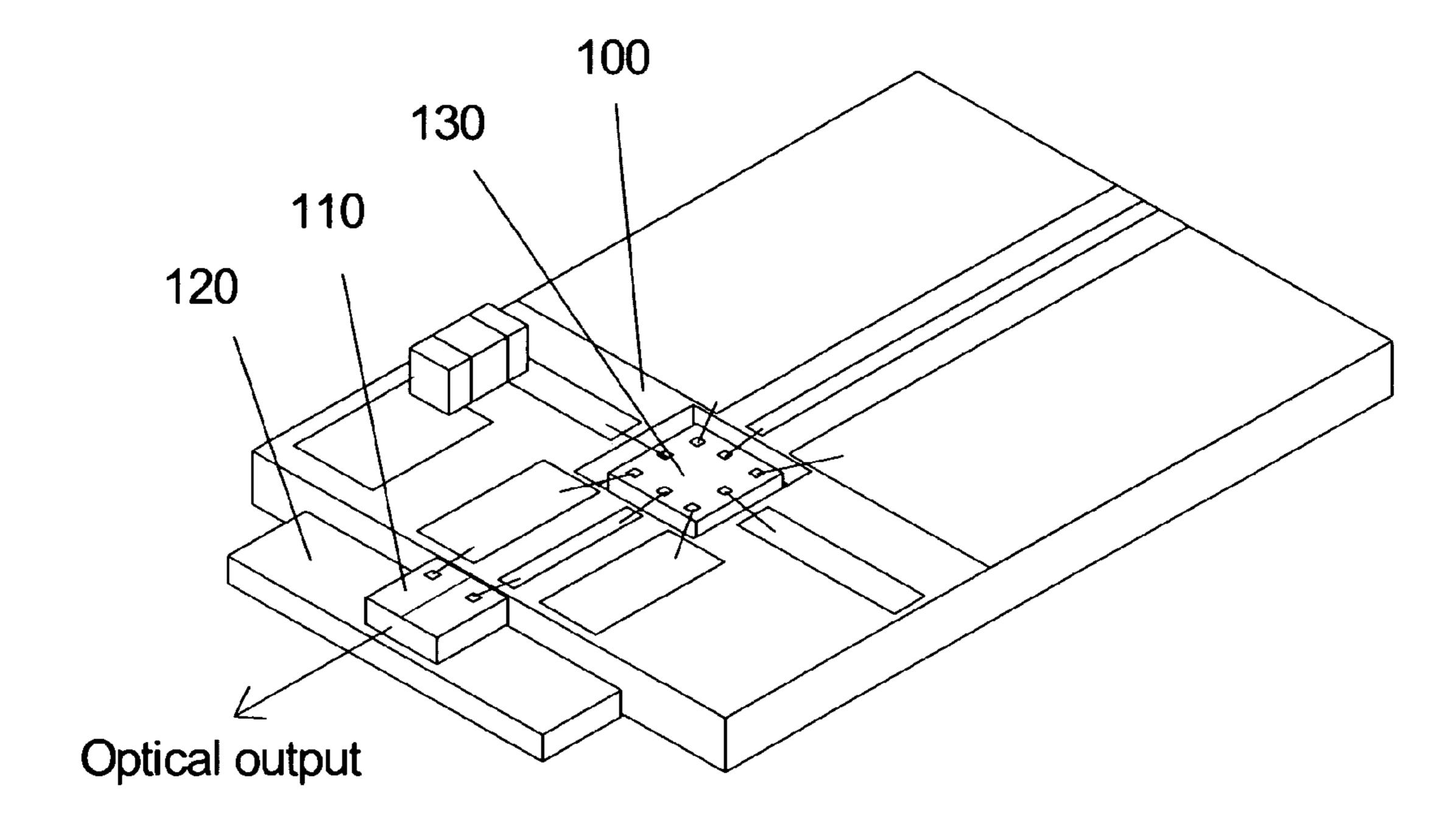
Figure 2: Assembly with transducer and micro-mirror on a mounting plate
