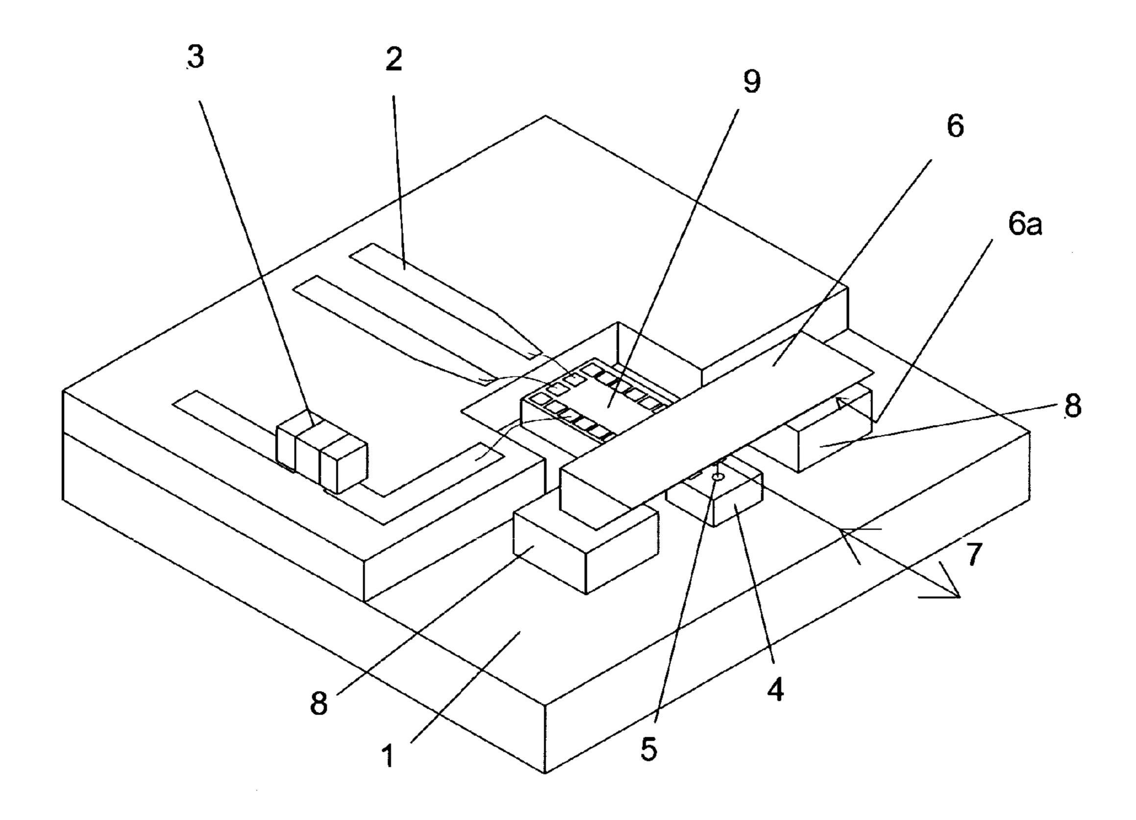
Figure 3: Assembly with standoff parts with a angled mounting surface
