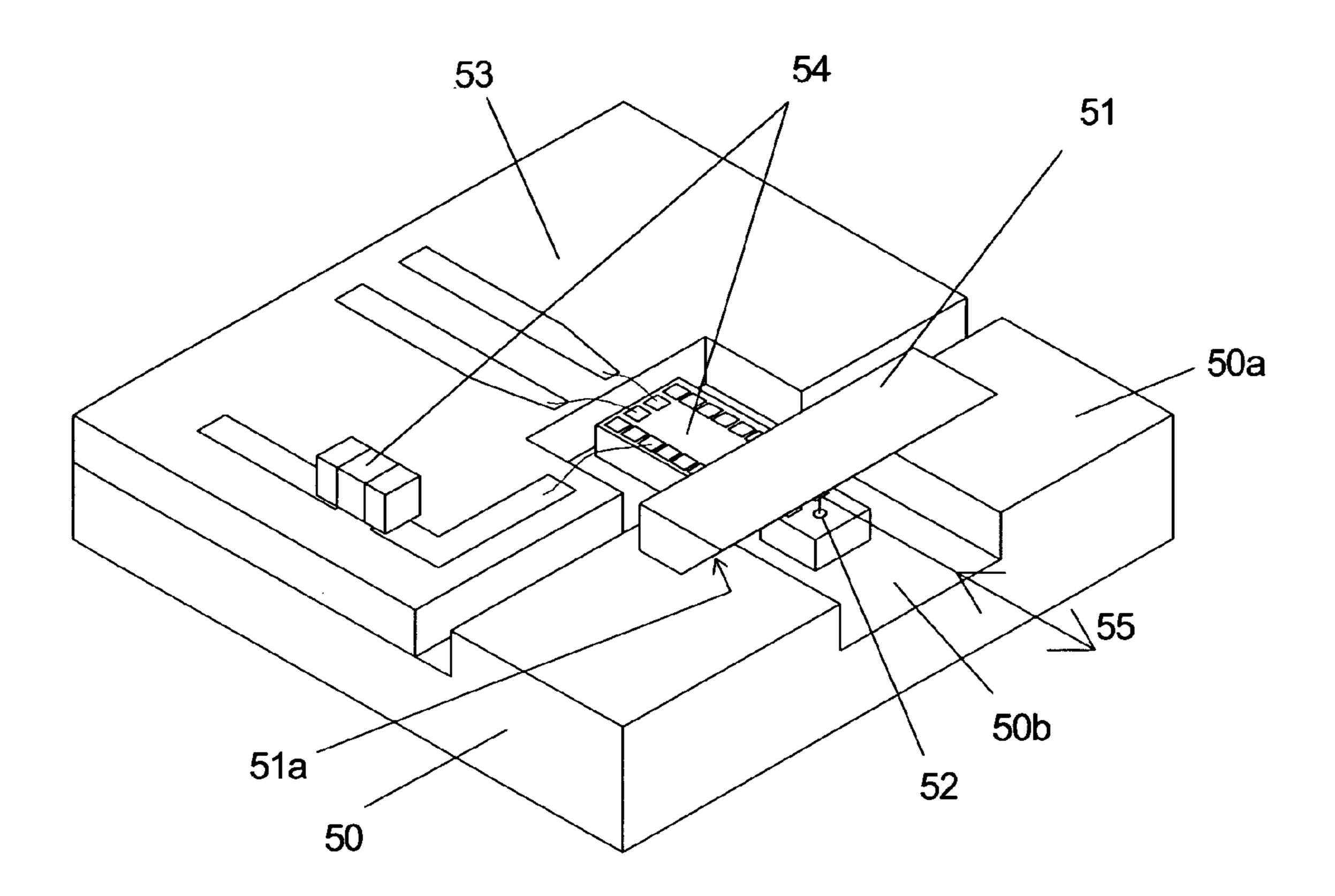
Figure 8: Assembly with micro-mirror mounted on standoff parts
