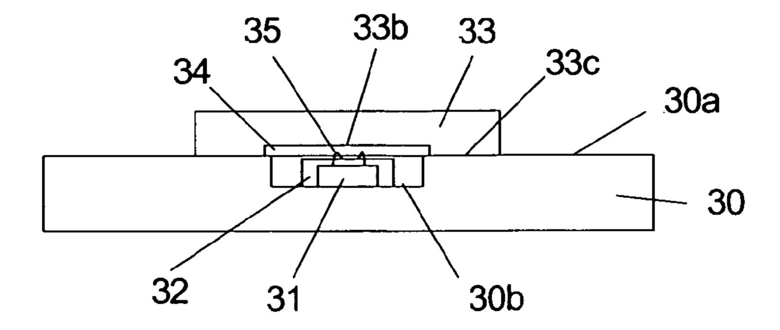
Figure 6: Bottom View of micro-mirror having a structured bottom side
