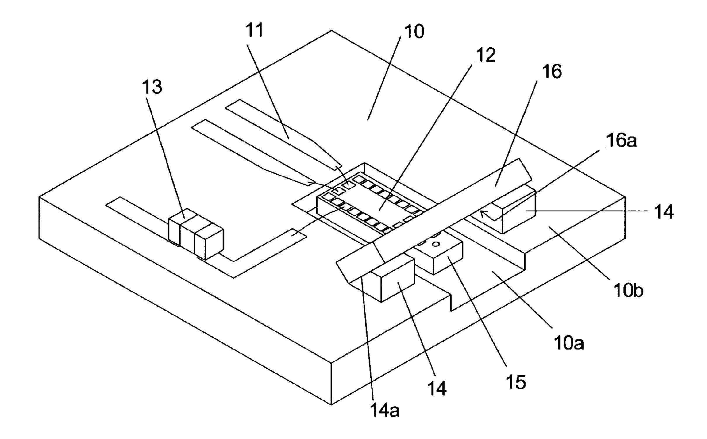
Figure 4: Assembly of a micro-mirror on a mounting plate with 3d structured top surface
