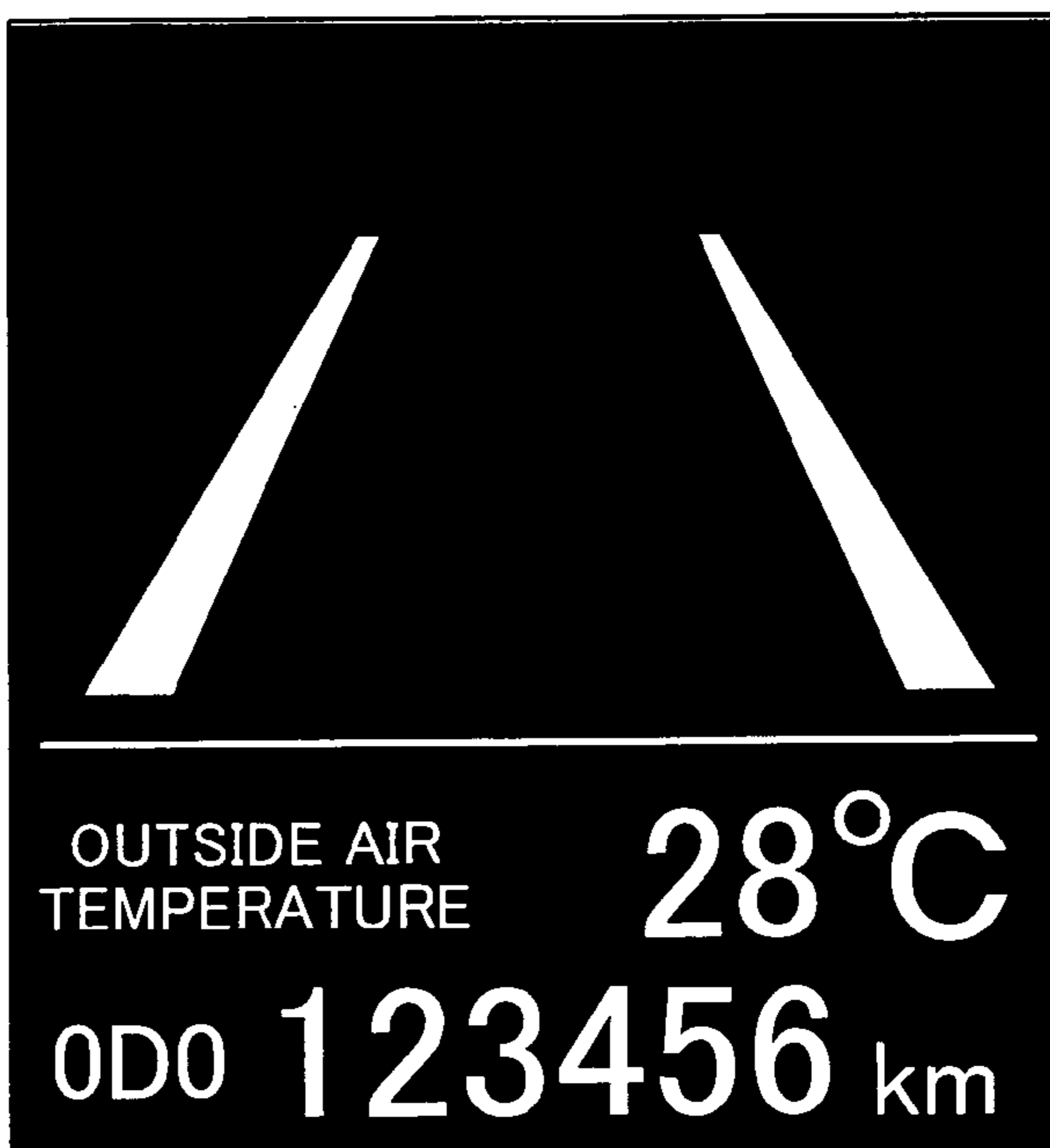
WHILE OPERATING (DETECTING WHITE LINE)
