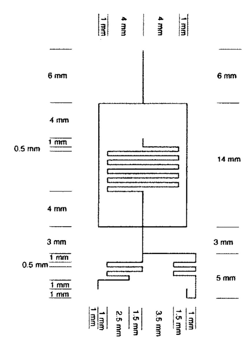
Drawing is on a 0.5 mm grid. All lines are 10 µm wide.
