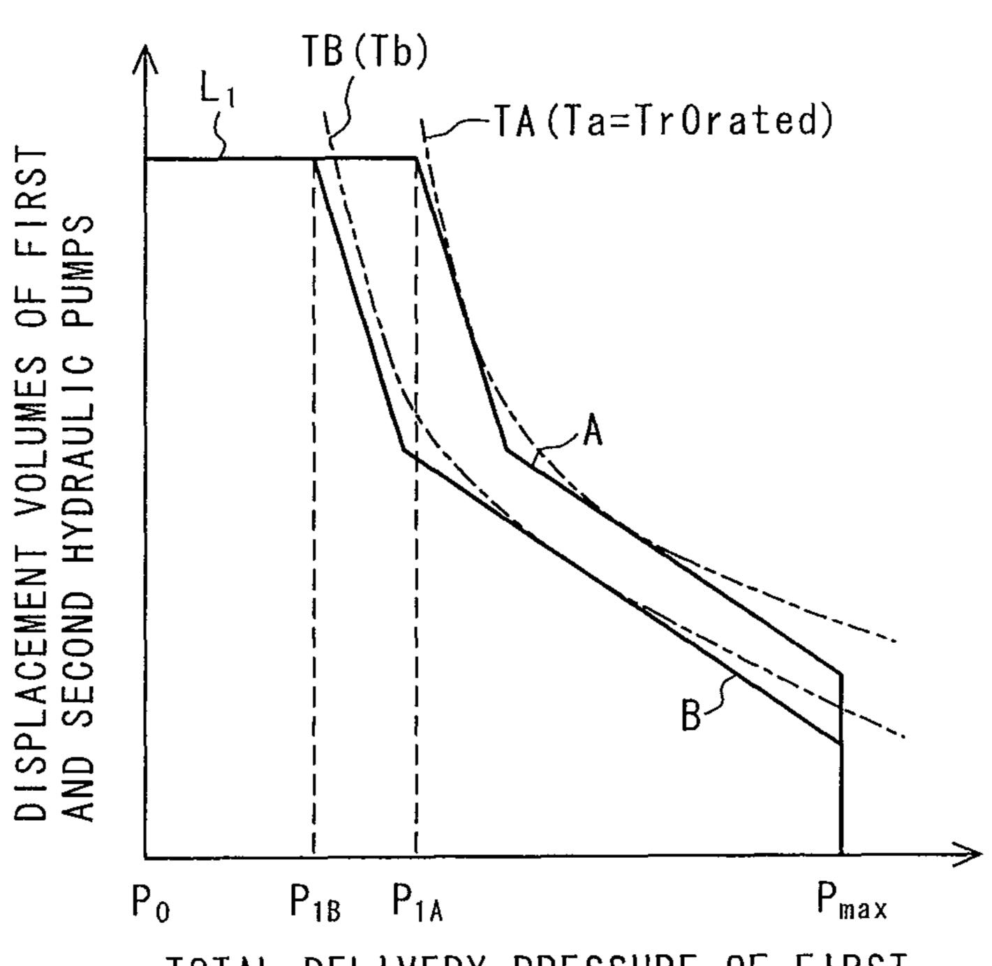
TOTAL DELIVERY PRESSURE OF FIRST AND SECOND HYDRAULIC PUMPS
