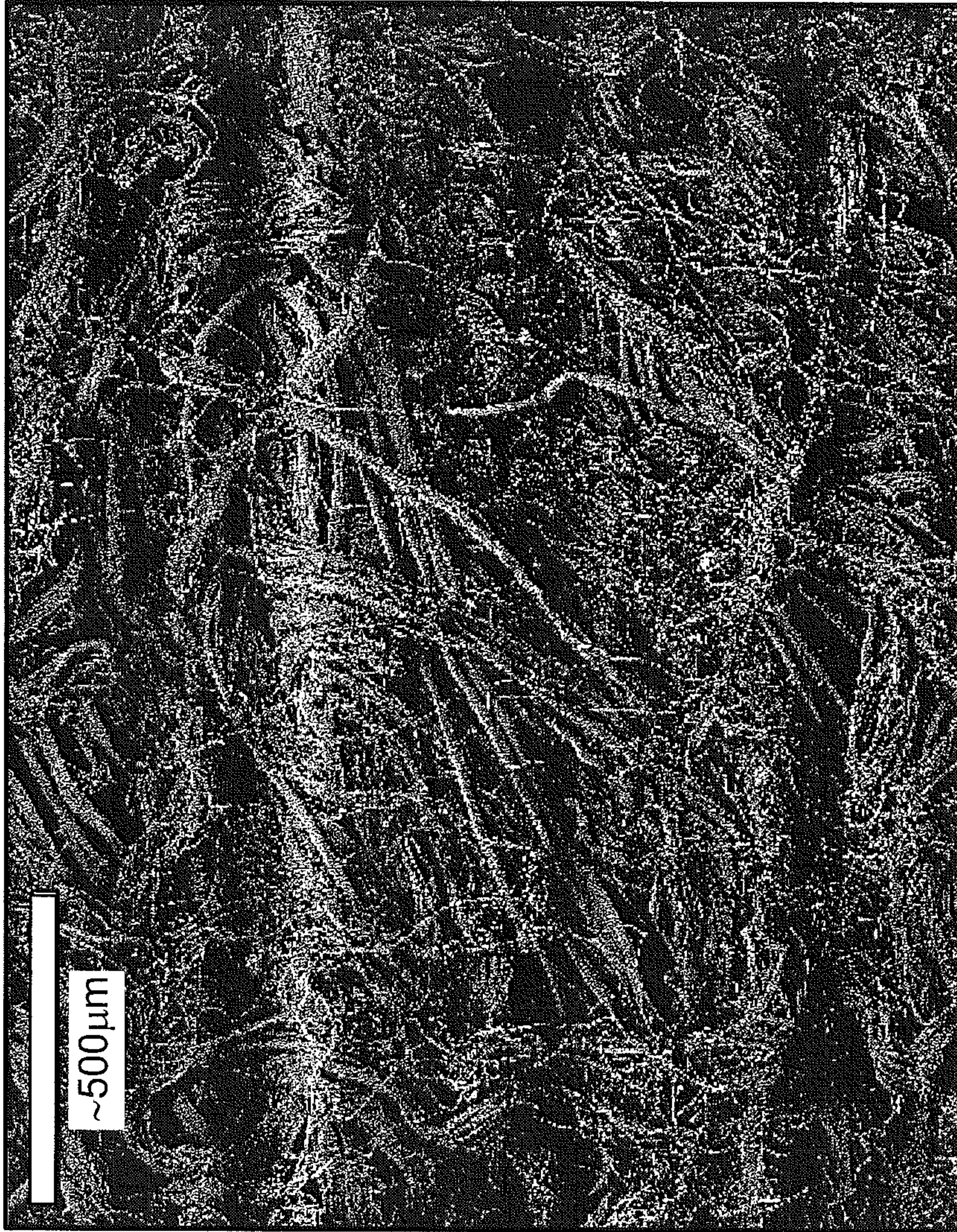
SEM Micrographs of Surface of an I-S Hydroentangled (Two Passes) and Dyed Spunbonded Fabric with Fibers Almost Completely Separated
