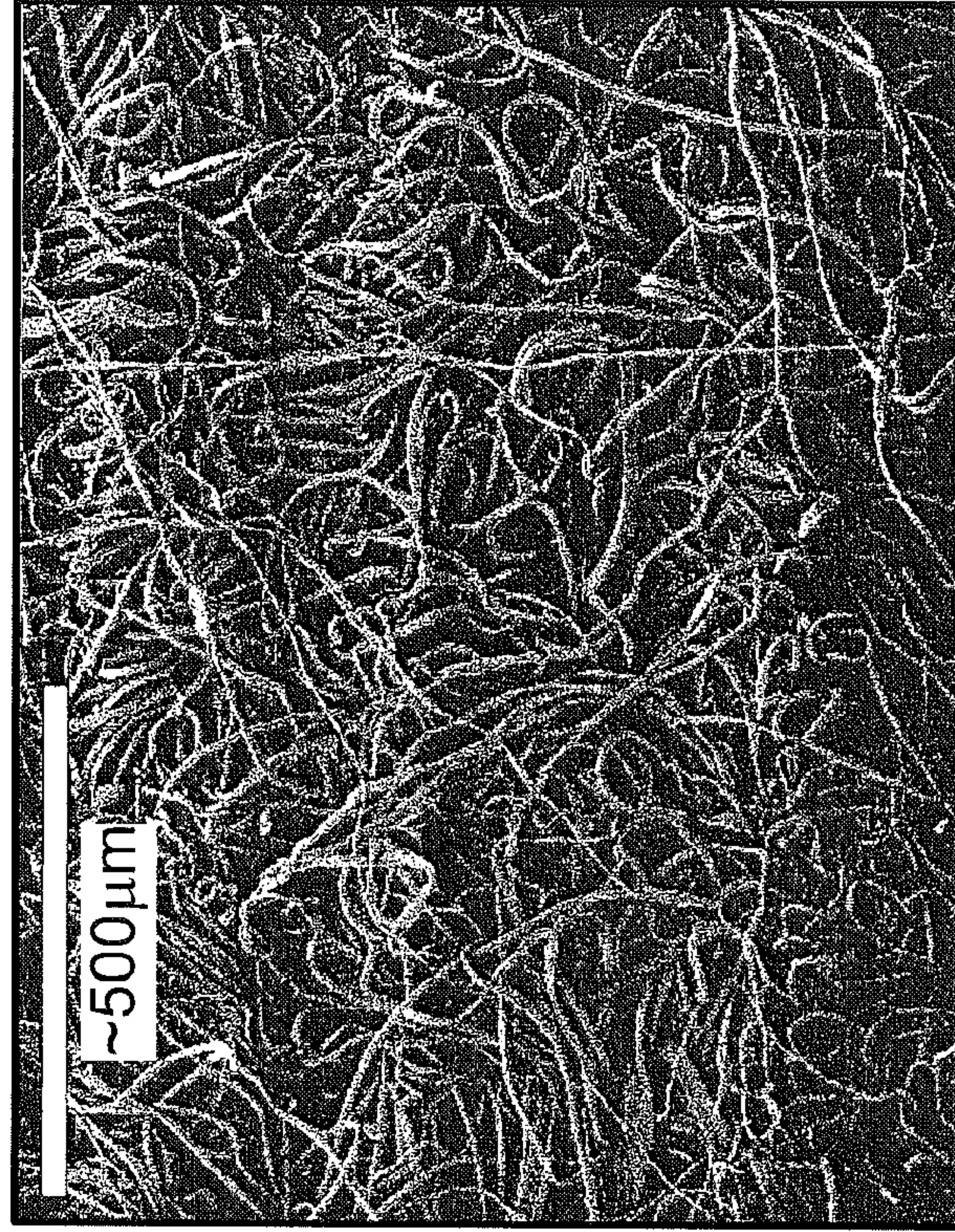
Hydroentangled and Fractured 100 gsm
